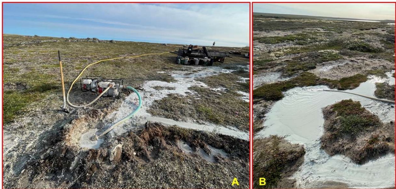
Figure 19. Photo of 24PB099 A) pumping drill cuttings, and B) discharge of drill cuttings into a depression.
