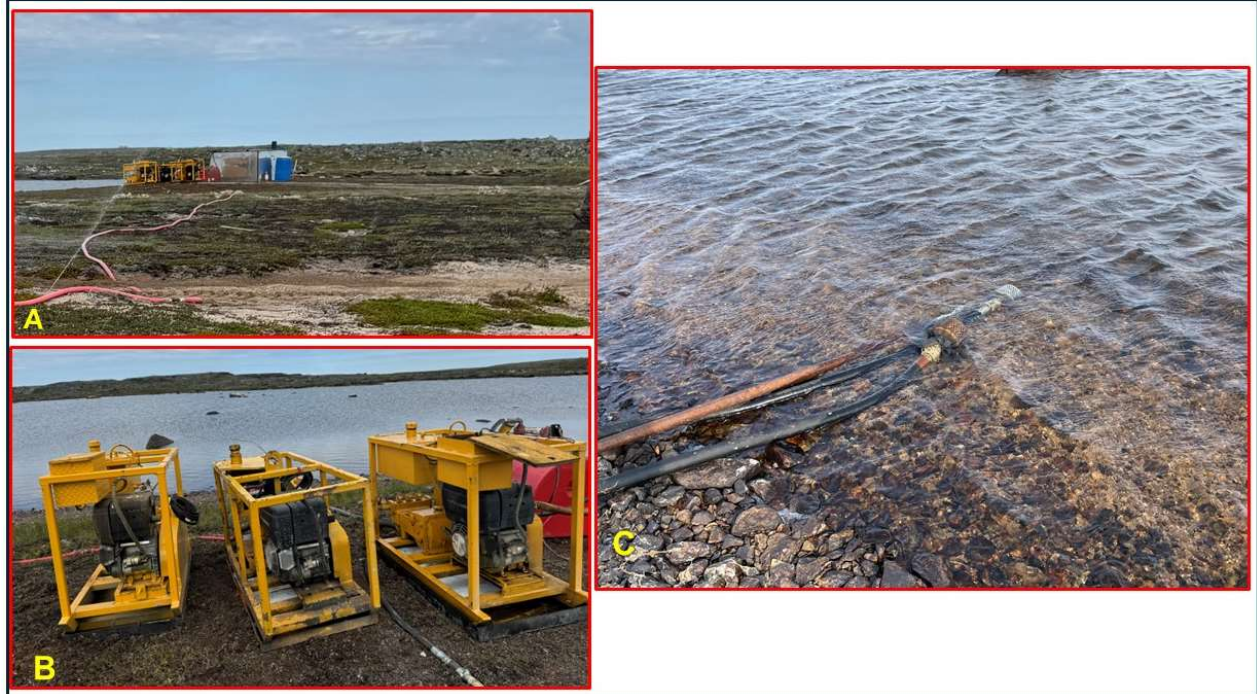
Figure 52. A) Photo of water pumps at site for DDHs 24PB099, 24PB101, 24PB103A and 104A, B) photo showing detailed view of the pumps, and C) photo of the pump's intake hoses with filters.
