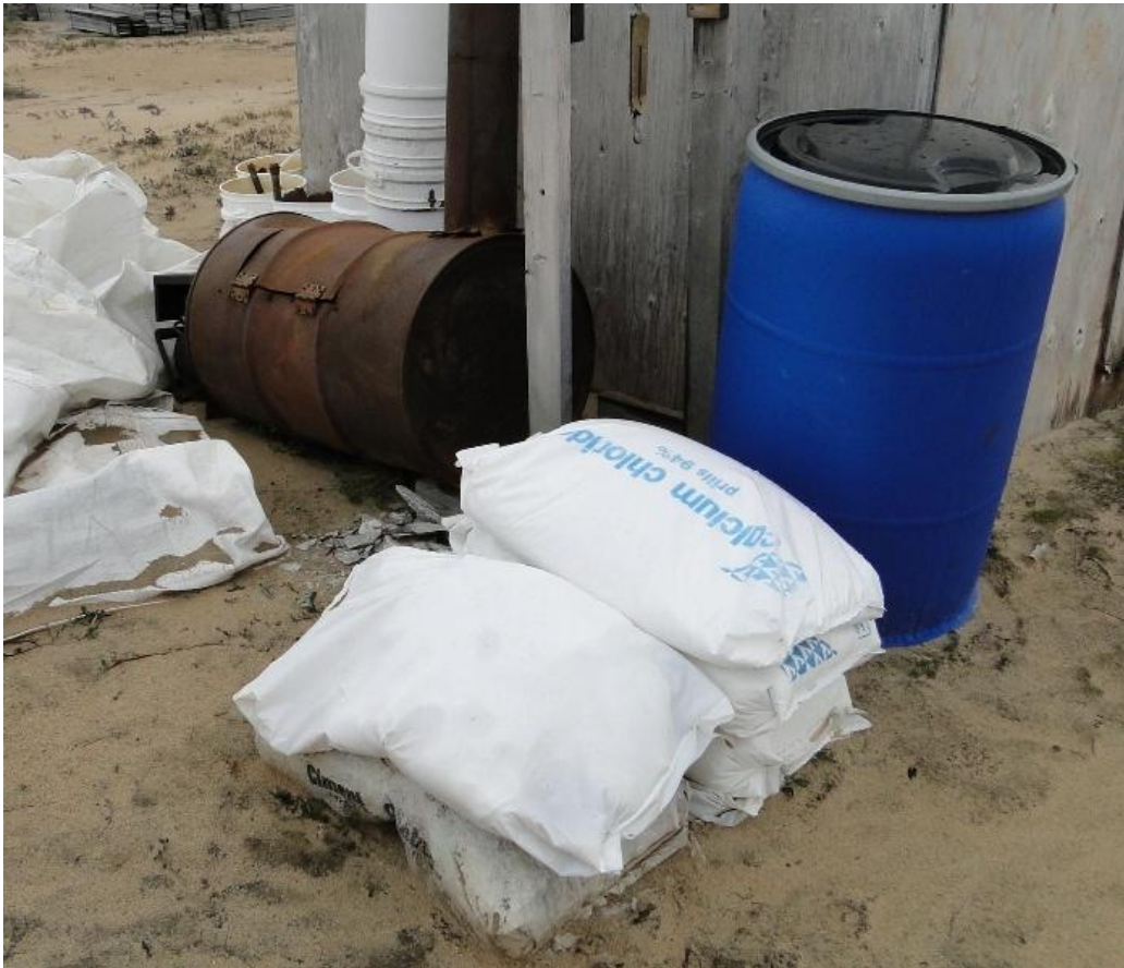
Figure 12. Salts stacked outside without containment.
