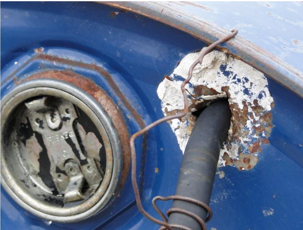
Figure 8. Incinerator Barrel - hole cut for hose.
