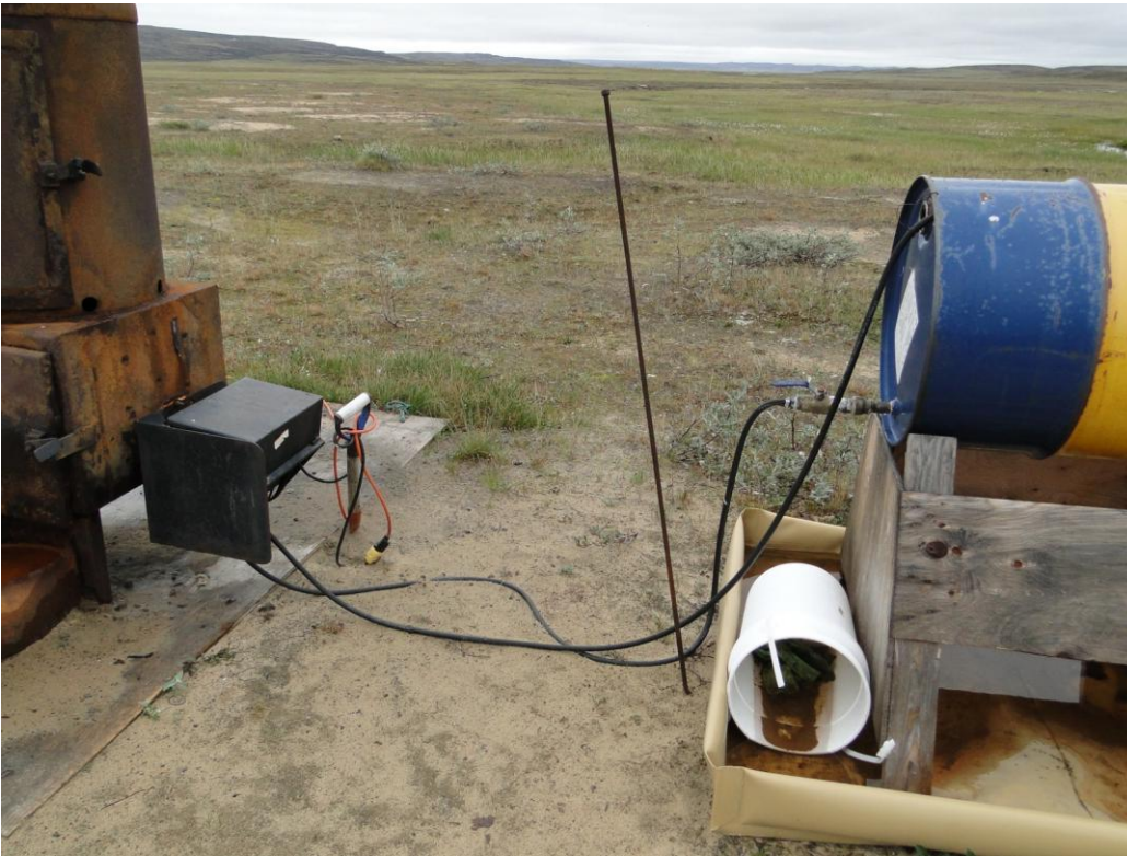
Figure 7. Incinerator barrel - berm full in low corner.
