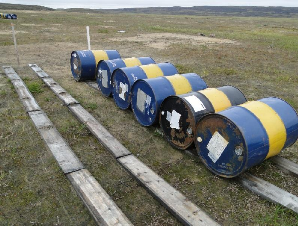
Figure 5. Full barrels, no containment.
