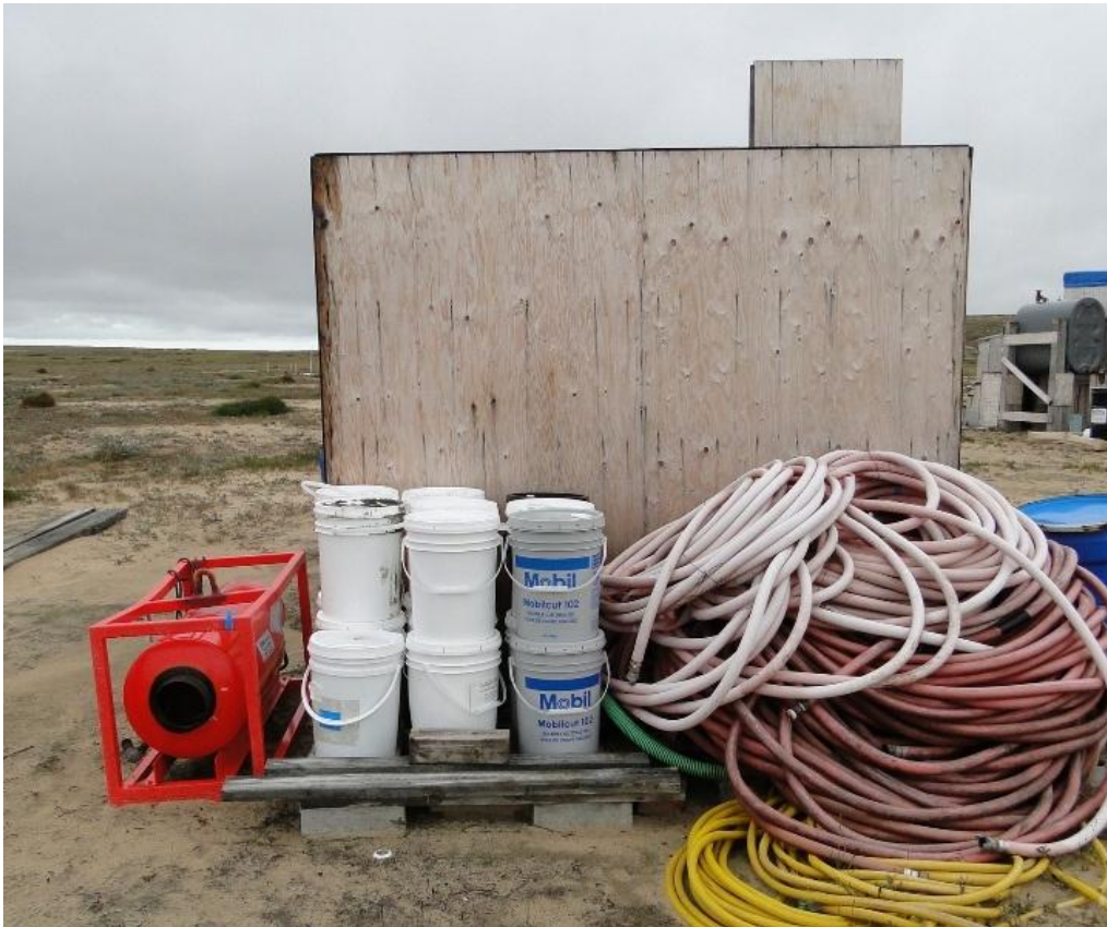
Figure 11. Oils stacked outside without containment.
