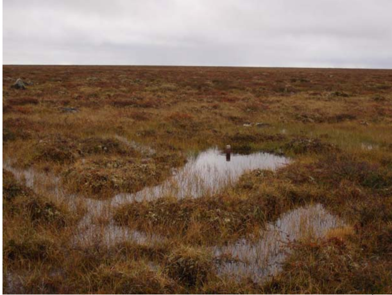
Figure 6. Visit to TUR-001 after the drilling completed on June 11 th . In the center of the image drill casing with a cemented cap is visible.
