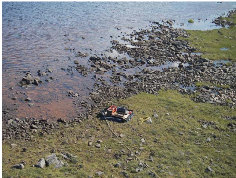
Figure 13. Aerial overview of the water pump and the hose supplying water to TUR-004. The pump is set up on a platform and protected by a berm.
