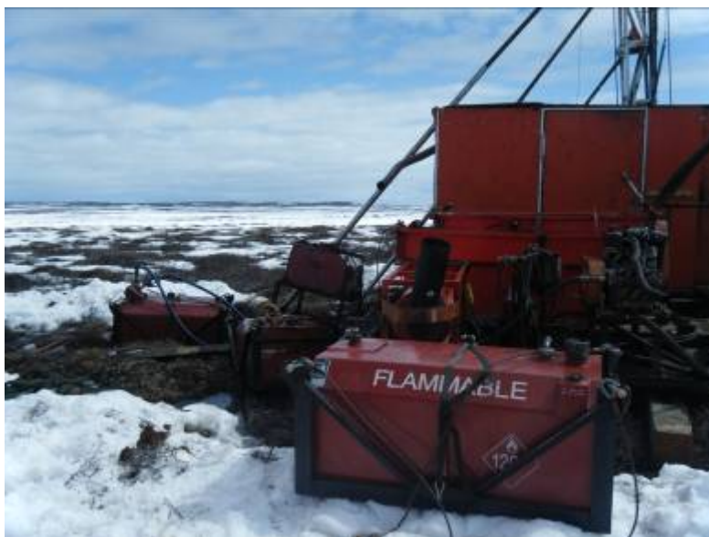
Figure 11. Overview of drilling in progress at TUR-006. All fuel is stored in double-walled metal containers.
