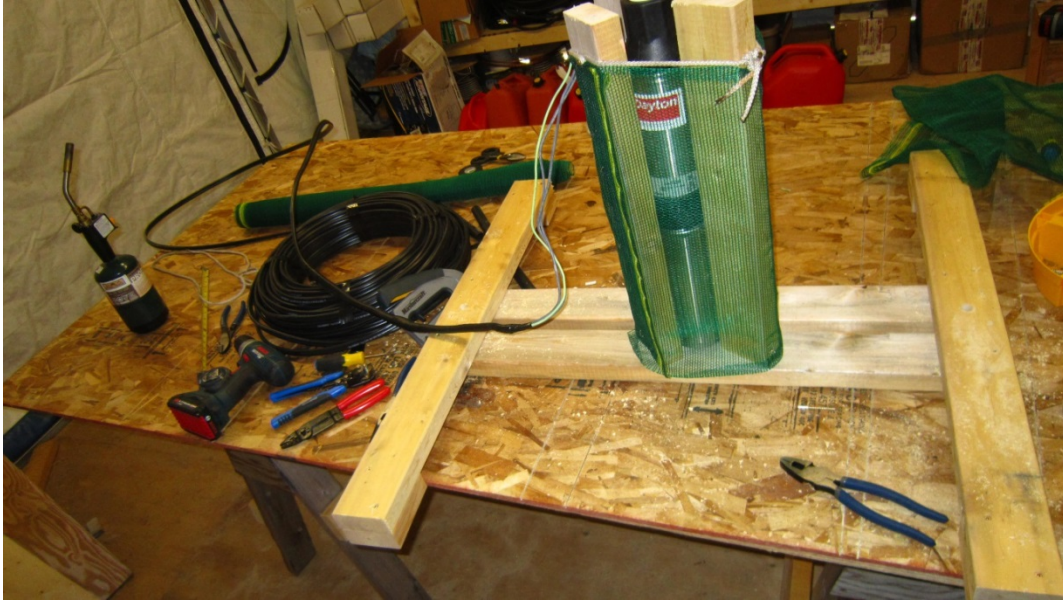
Figure 5: Photograph showing the new electric pumping system that eliminated the gas driven unit.
