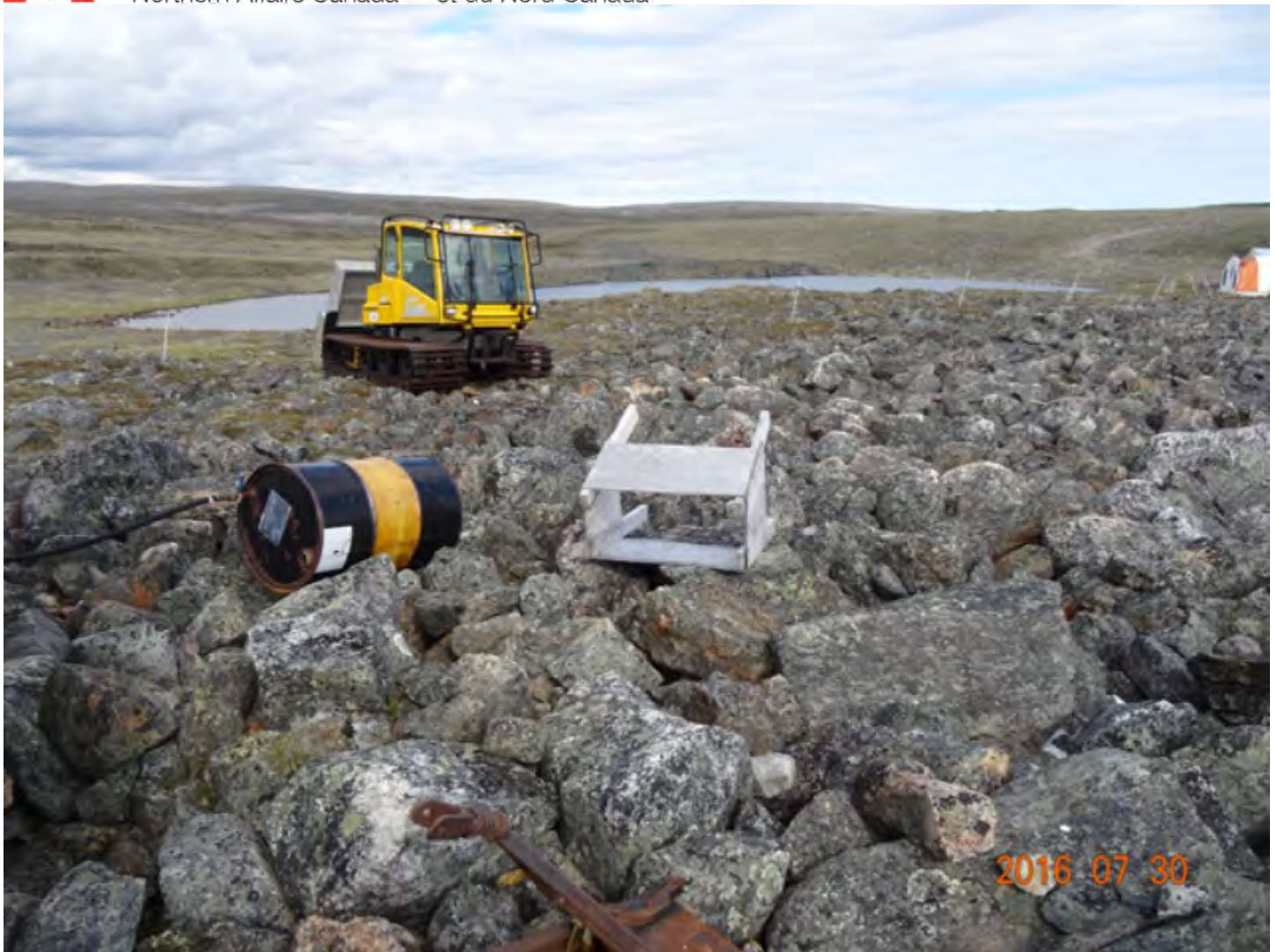
Figure 47 Challenger and barrels at camp (2) – No secondary containment
