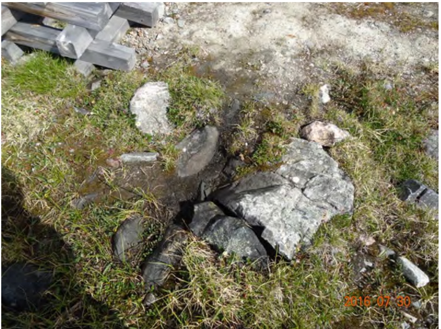
Figure 42 Hydrocarbon contaminated soils behind workshop
