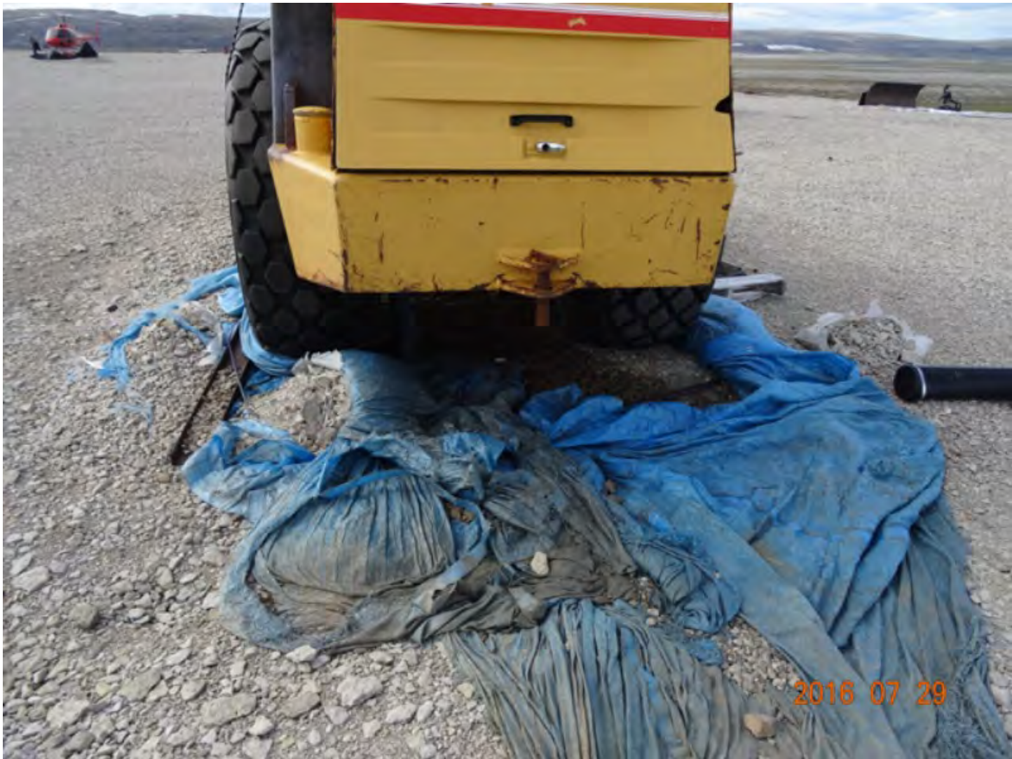
Figure 2 Roller on airstrip - note oil leaking from under carriage
