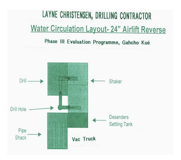
All drill fluid flows from drillhole to drill, to shaker, to desanders and back down drillhole. All drill fluid is recirculated. Fines are hauled away from settling tank by vac truck.
