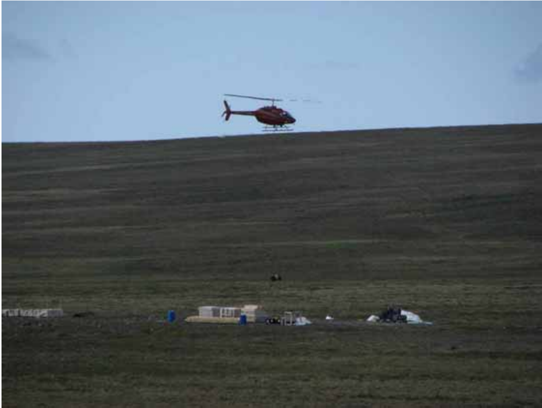
Figure 4: Slinging fuel drums to the containment berm at the Thom Lake fuel cache.
