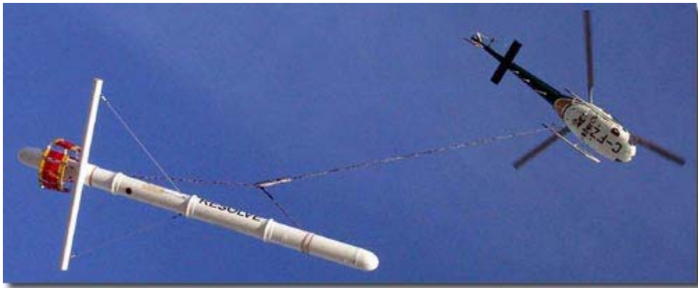
Figure 5: Fugro Airborne Surveys RESOLVE™ survey set-up (photo taken from Fugro Airborne Surveys website).
