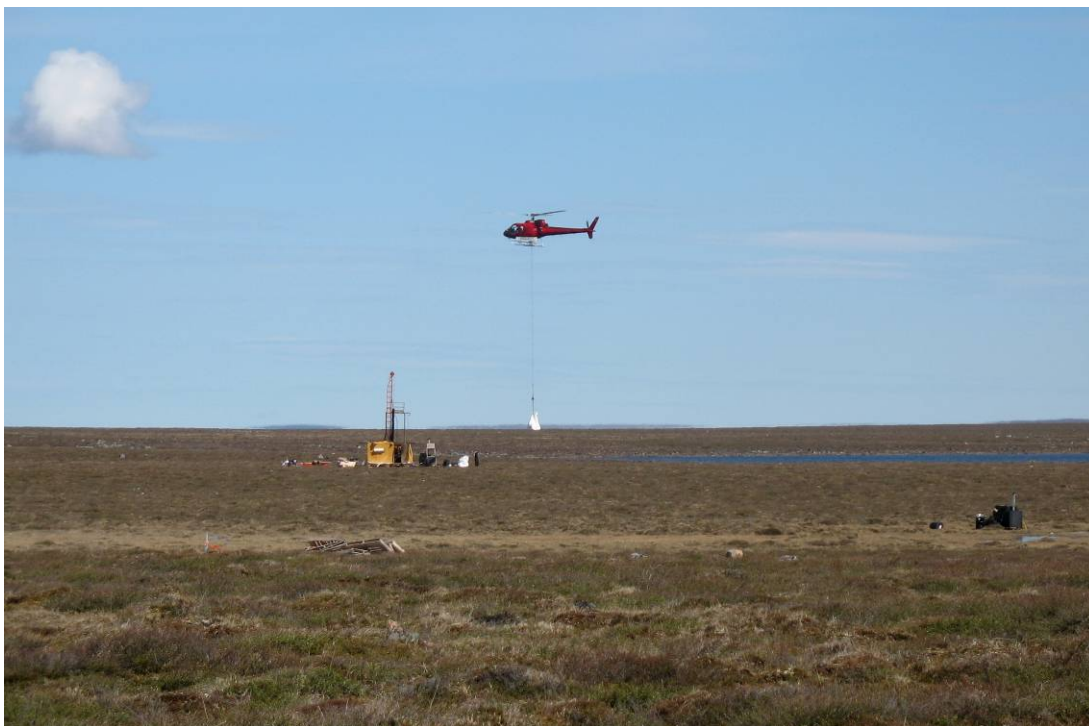
Figure 10: Example of drilling operations. The helicopter is slinging salt to the drill in a nylon ore bag. In the foreground is the water supply pump as well as a pile of pallets used for cribbing the drill floor.
