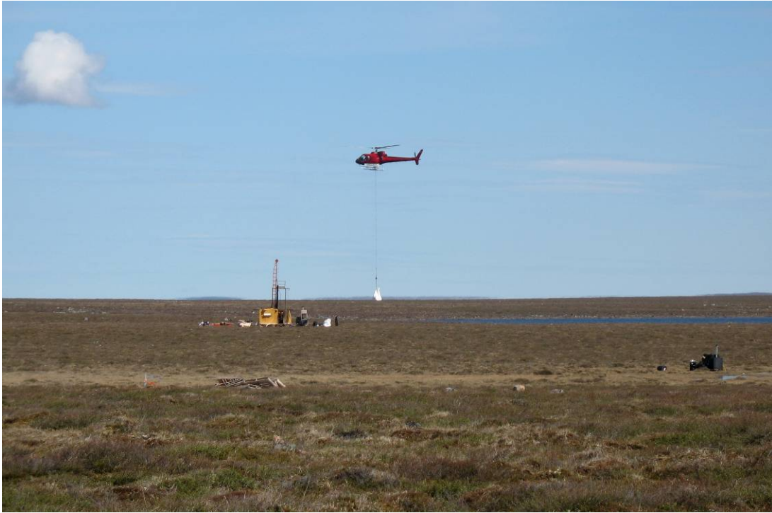
Figure 5: Example of drilling operations. The helicopter is slinging salt to the drill in a nylon ore bag. In the foreground is the water supply pump as well as a pile of pallets used for cribbing the drill floor.
