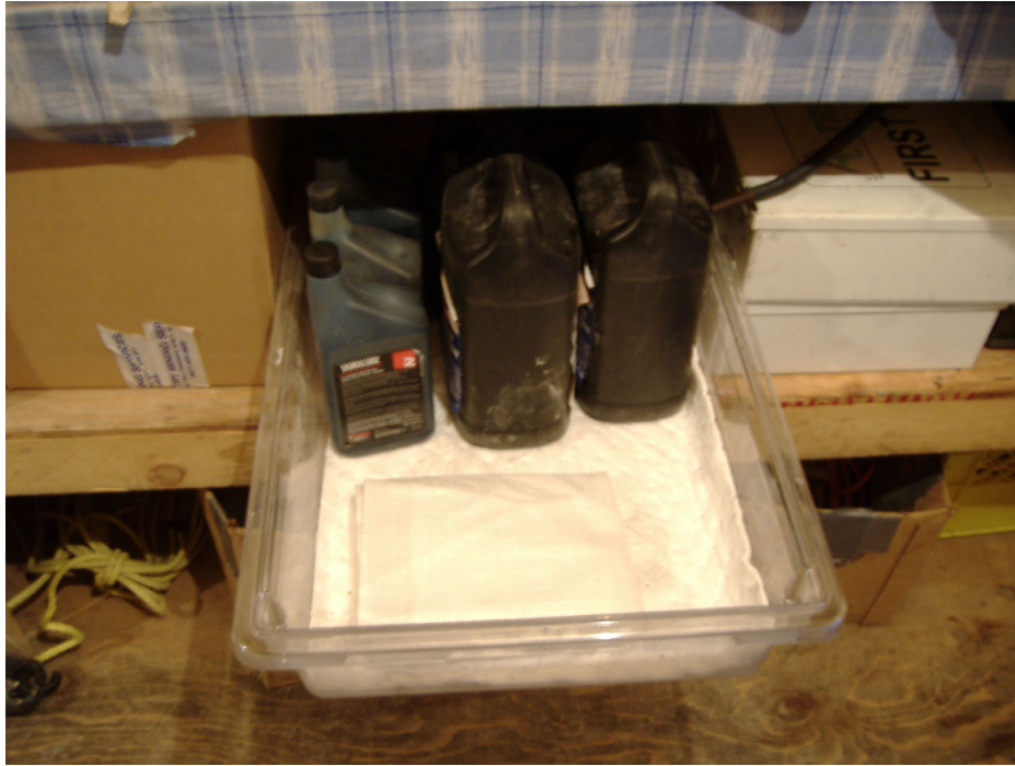
Secondary Containment Measures Implemented for the Storage of Products In the TV Tent
