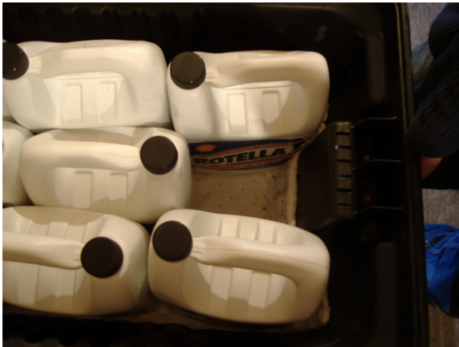
Secondary Containment Measures Implemented for the Storage of Products In the TV Tent
