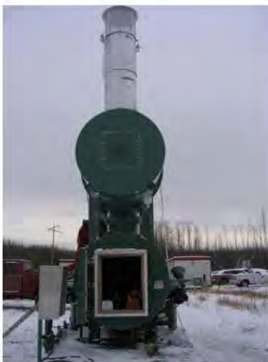
Figure 2.2 Typical Controlled Air Dual Chamber Incinerator
