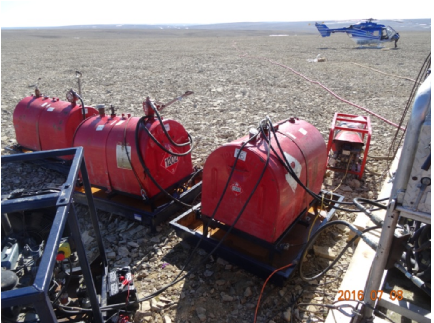
Figure 8 Fuel storage all double walled transport containers
