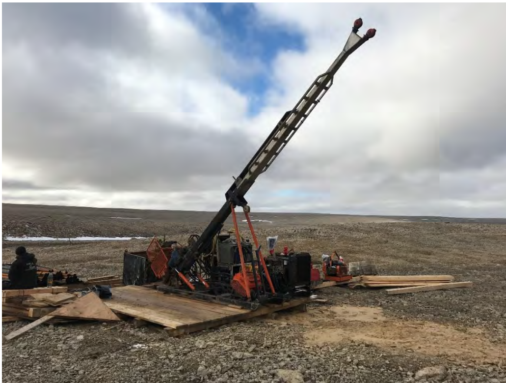
Photo 17: Drill Pad AB18-09 (drill stored on site – materials subsequently tidied up, all fuel & oil drained from equipment)
