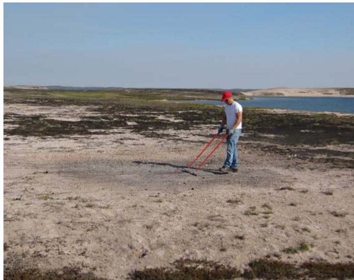
Figure 7. Demonstrating magnetic sweeping after burning to remove nails, screws, and other metals from the ground after burning was completed. July 2013.
