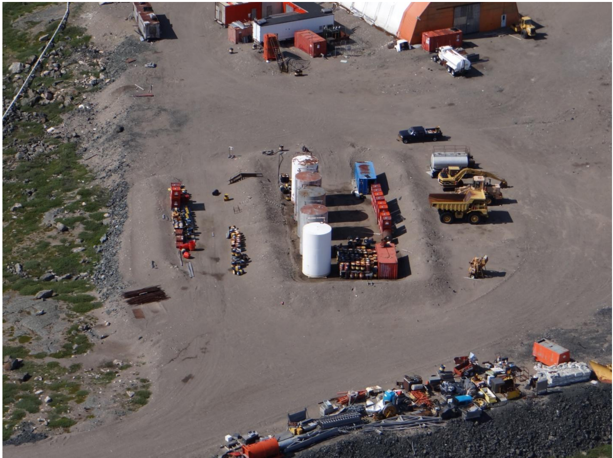
Figure 5. Many barrels have been moved into the tank farm berm and the lined storage area beside it.
