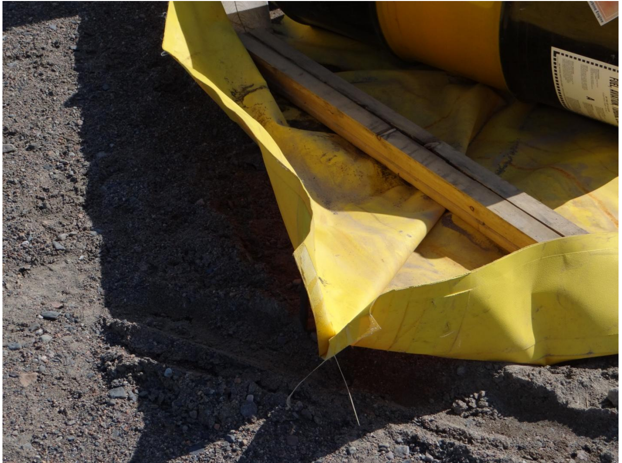
Figure 9. The berm containing MMG's fuel is ripped.
