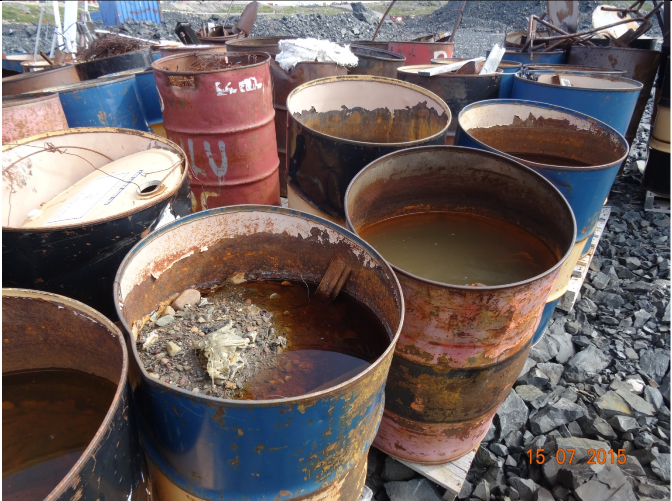
Description: Waste barrels at the mine storage pad. Several barrels of soil (possibly contaminated) and metal waste.
