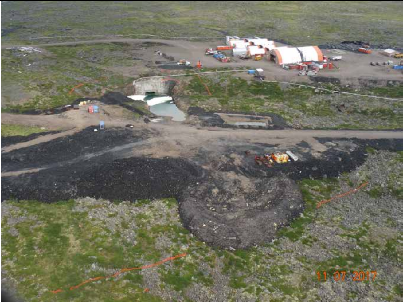
Description: Water ponding in the portal is near to the road.
