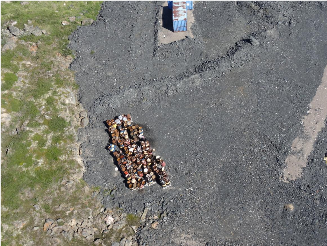
Figure 3. Barrels of waste on Mine Waste Pad. Staining noted.
