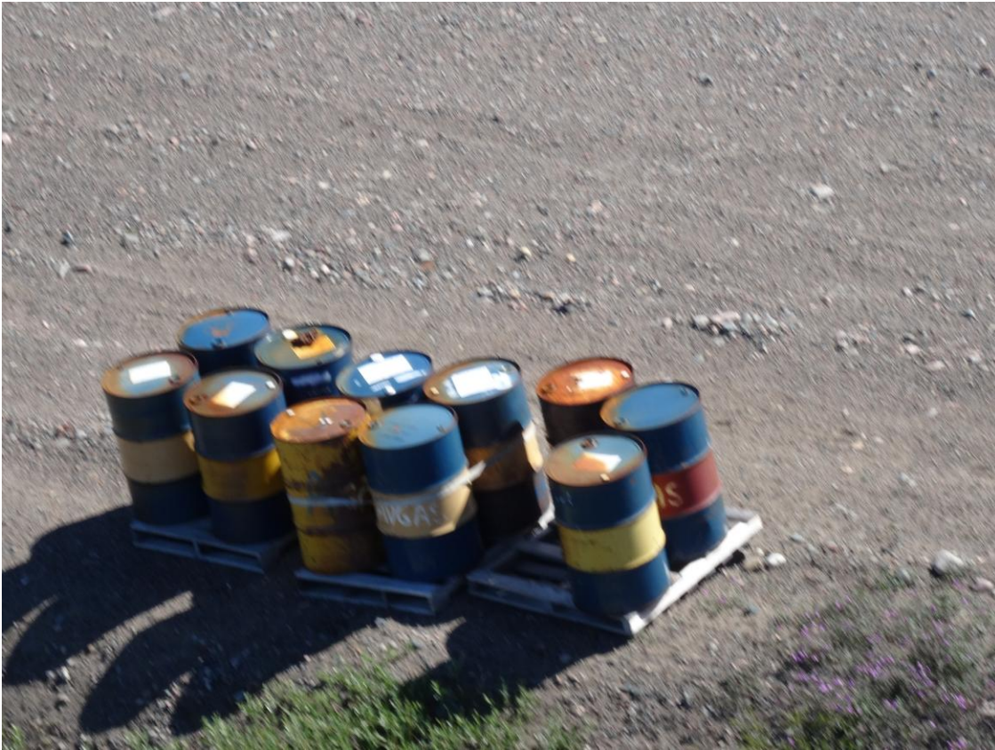
Figure 15. Barrels noted on pallets (without containment) on the roadside near the airstrip.
