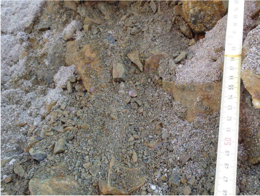
Photo 2: Orange strongly oxidized rock (some sand also present)
