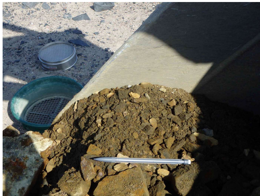
Photo 2: Orange strongly oxidized rock sampled with excavator bucket
