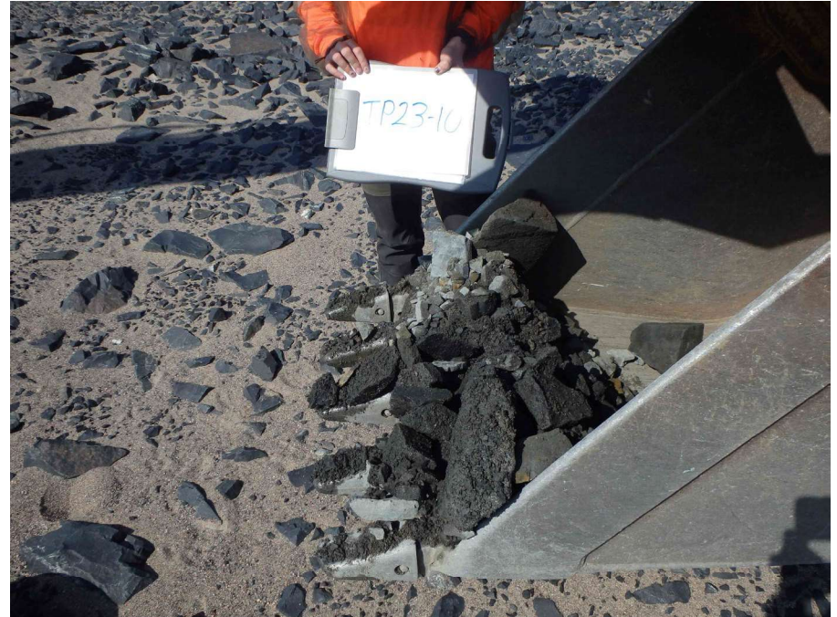
Photo 2: Grey metabasalt sampled with excavator bucket
