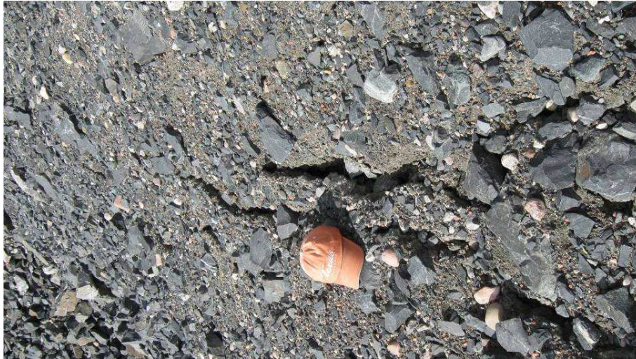
Slump Cracking Downhill Side – 2010
