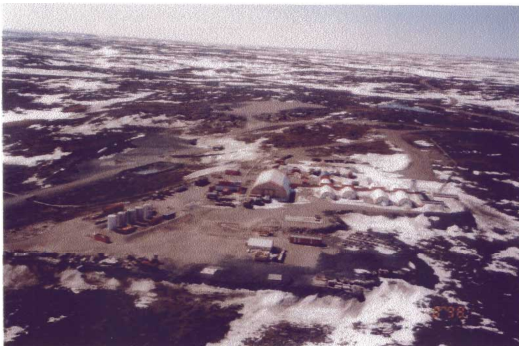
Photo 1 Ulu Project Camp looking from the northeast. Laydown area in foreground, fuel tank farm on left, underground surface sump - middle left, weatherhaven camp and ore storage pad (center above camp).
