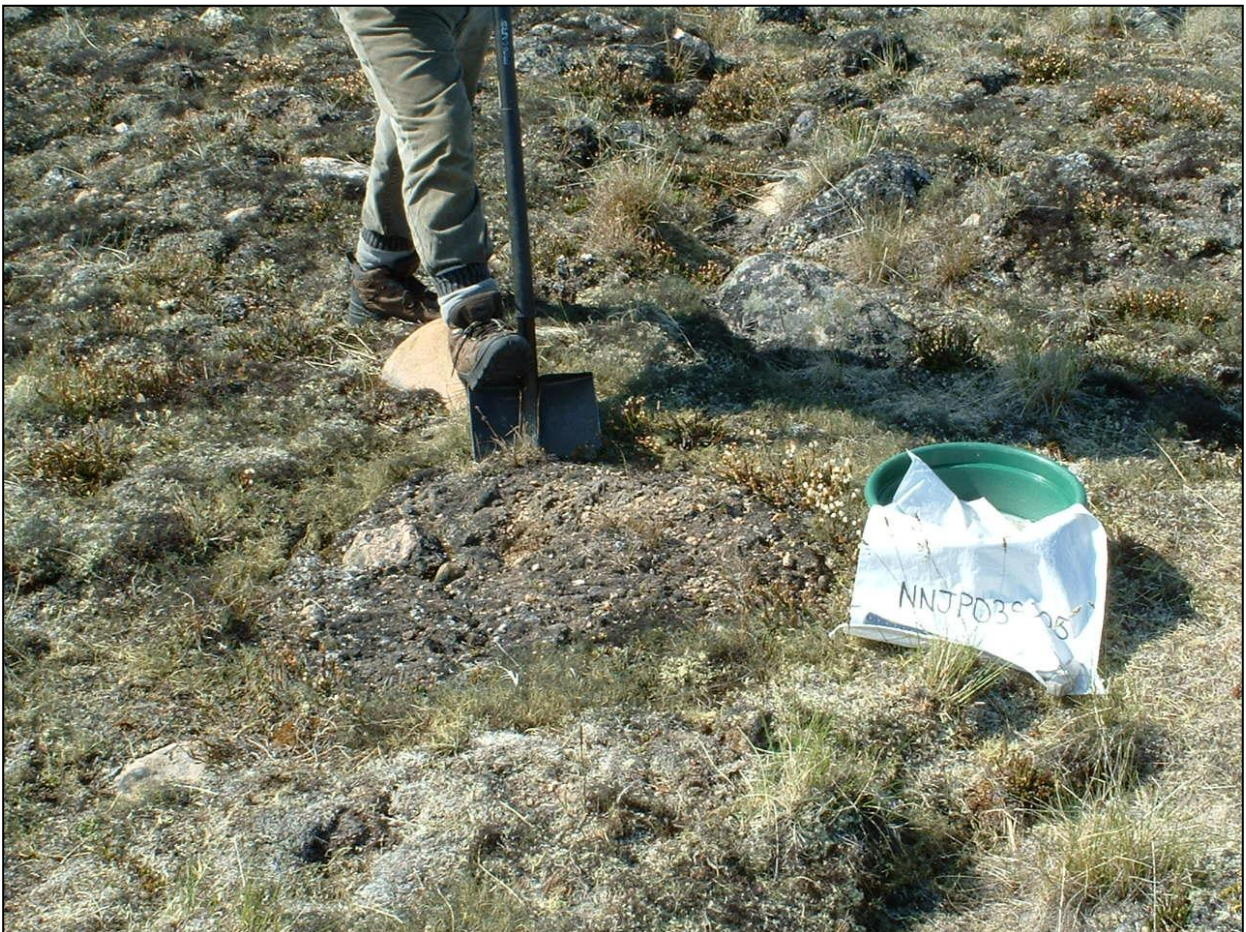
Figure 3. – Example of sampling a mudboil (till)
