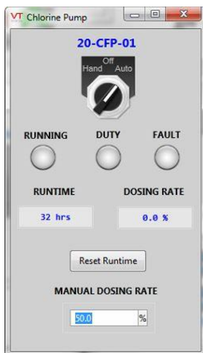
Figure 28 Chlorine pump display on the HMI
