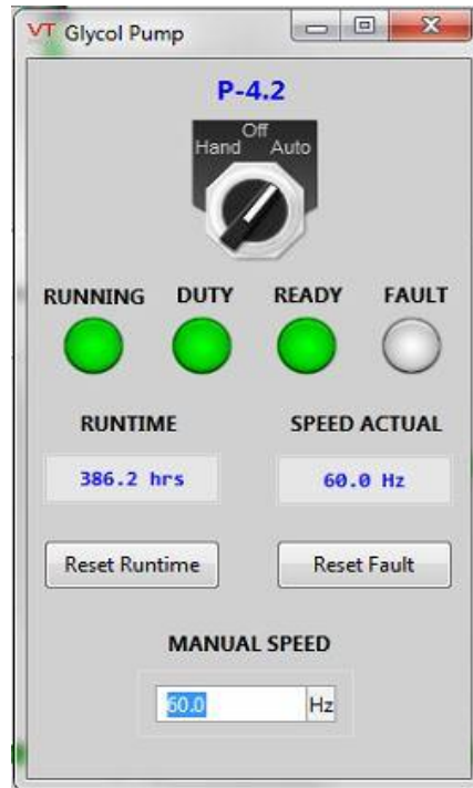
Figure 21 – Glycol Circulating Pump Popup Screen
