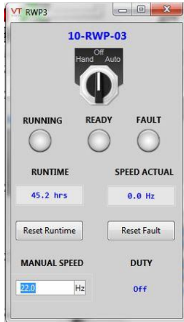
Figure 8 Raw Water Pump Popup Screen
