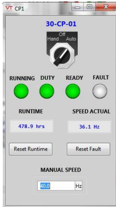
Figure 14 – Circulating Pump Popup Screen
