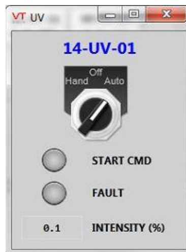
Figure 22 UV controls on the HMI
