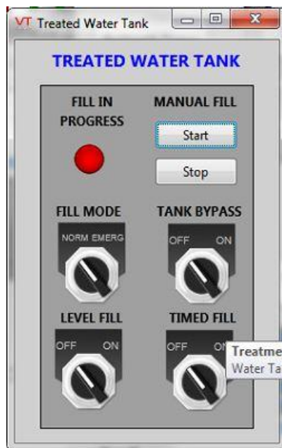
Figure 11 – Treated Water Tank Fill Controls
