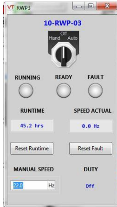
Figure 12 – Raw Water Pump Popup Screen
