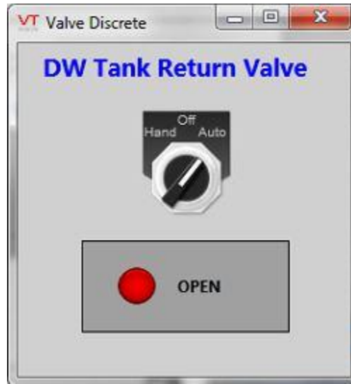
Figure 20 – DWT Return Valve Popup Screen
