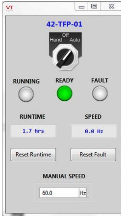
Figure 18 – Truck Fill Pump Popup Screen
