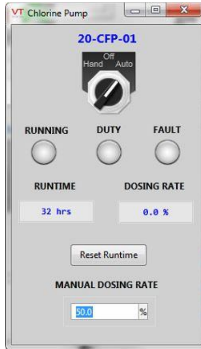
Figure 13 – Chlorine Pump Popup Screen
