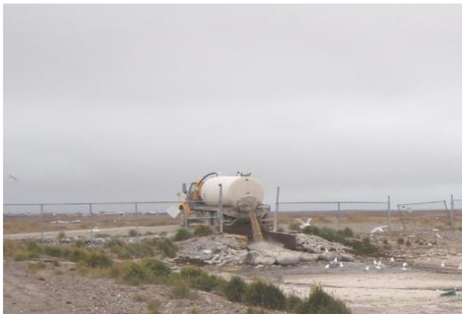
Raw sewage being dumped at truck off load point. Date: 9/10/2010
