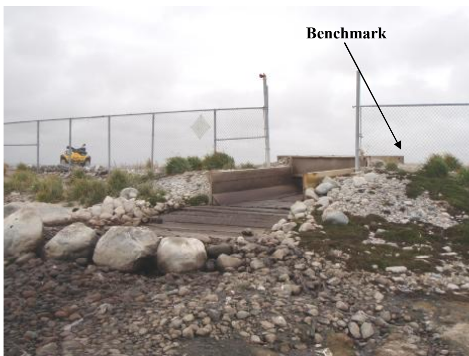
Monitoring Station ARV-8 Benchmark used to survey water level in Sewage Disposal. Facility Lagoon Date: 9/10/2010
