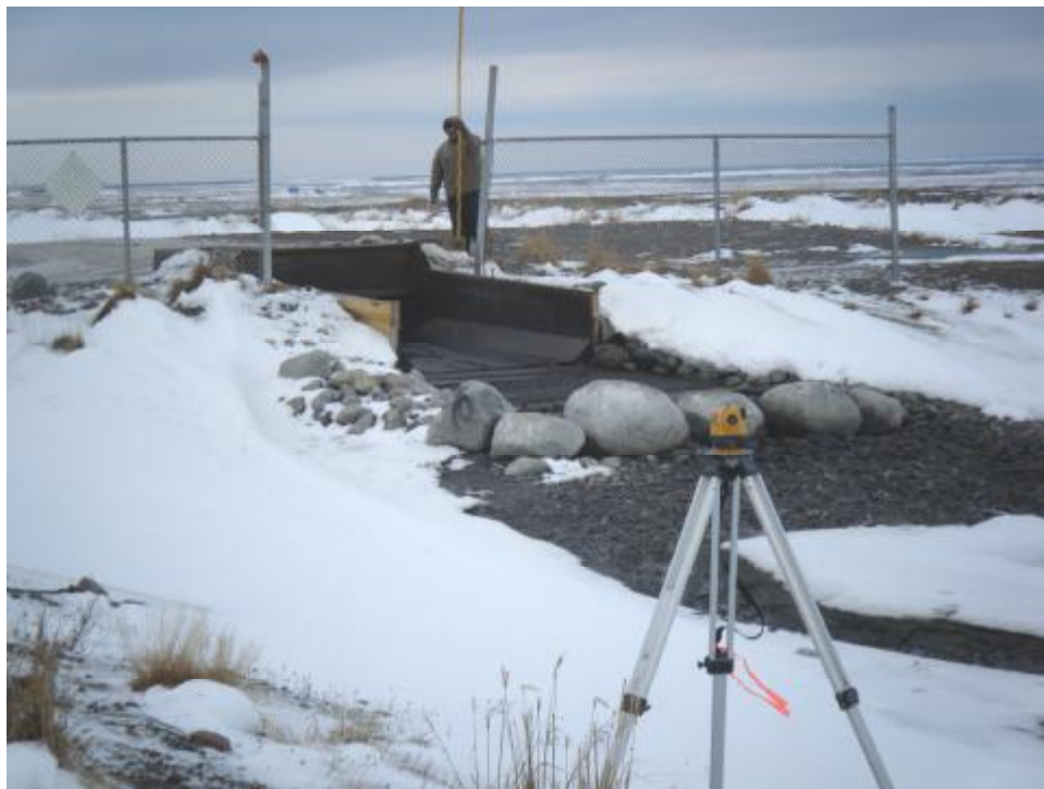
Level set up to survey benchmark and water level of sewage lagoon.
