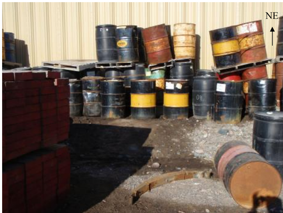
Hazardous Waste Storage Area Stained soil beside waste oil drums.
