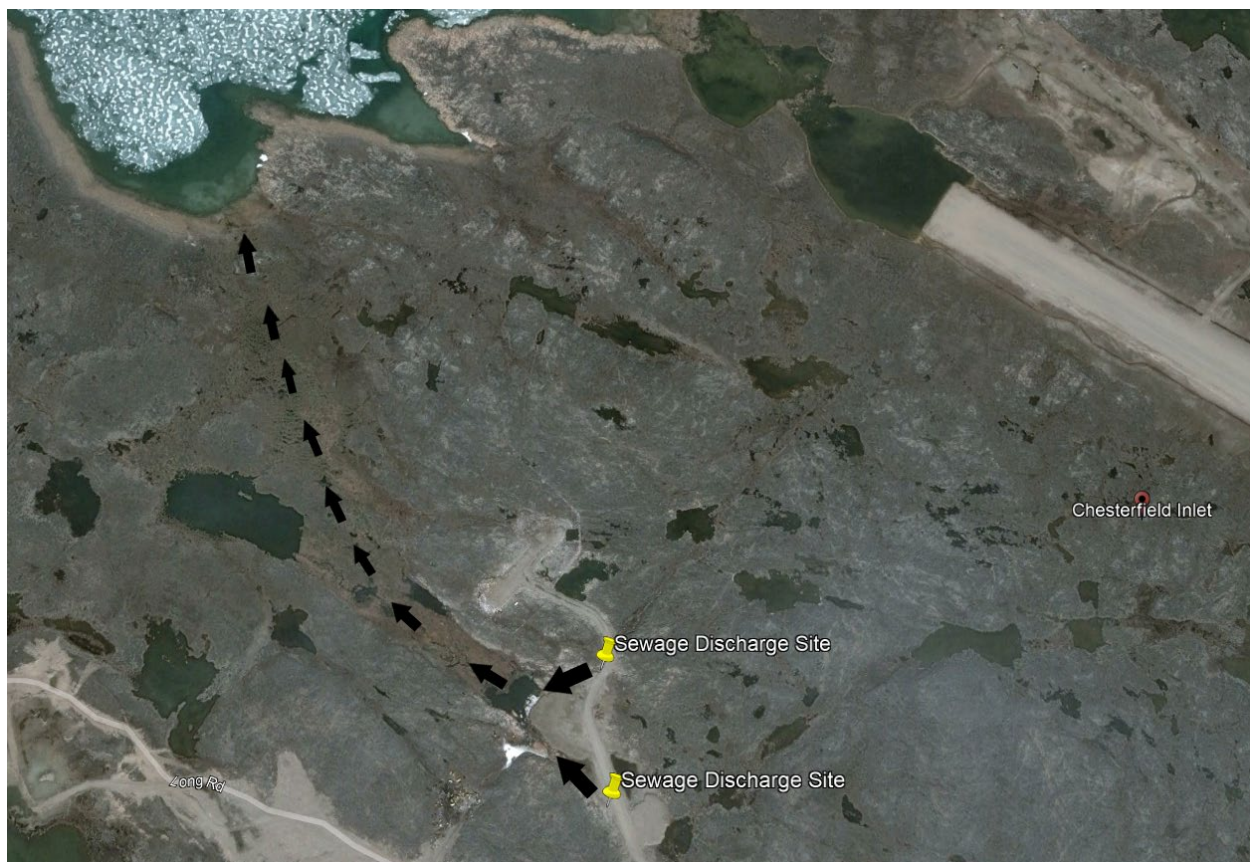
Figure 2 Effluent flow through the wetland treatment area
