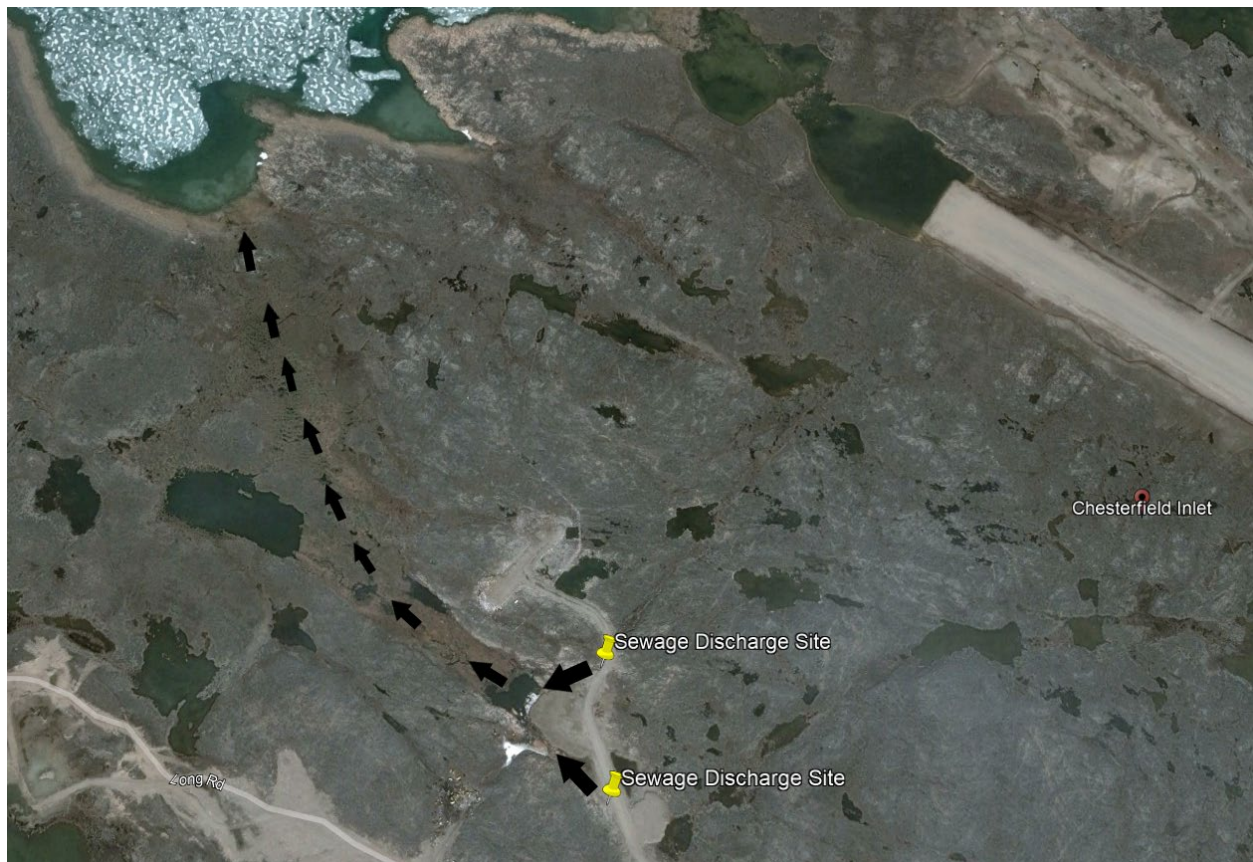
Figure 2 Effluent flow through the wetland treatment area
