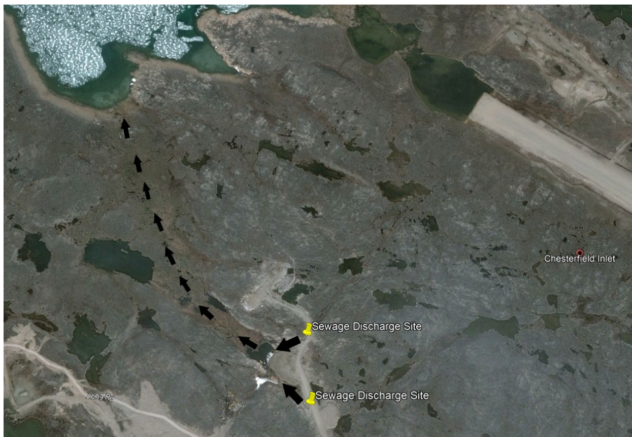
Figure 2 Effluent flow through the wetland treatment area
