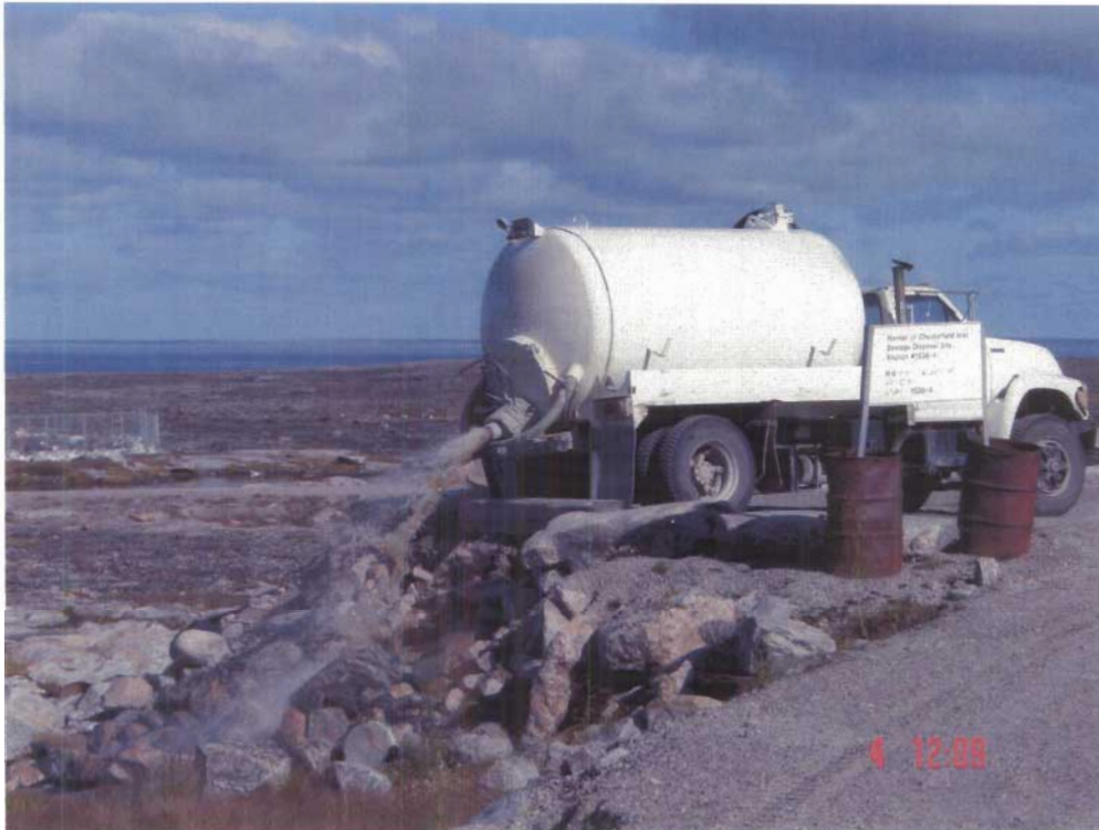
Photo # 7. Sewage truck shown discharging at Sewage Treatment Facility discharge structure with sign shown by truck.
