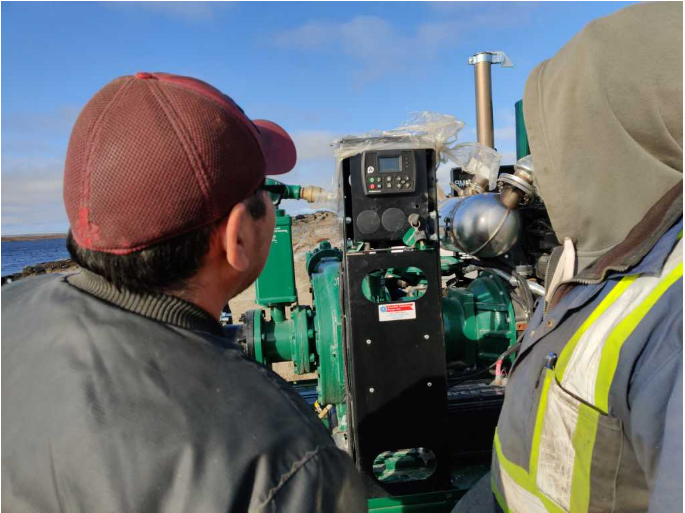
Photo 1:10 pm – Photo taken at pump at station 0+0000. Walkthrough of pump startup procedures with Don, Hamlet Foreman takes place with ICL’s mechanic. Factory-optimized operating speed and flow rate were discussed, along with pre-startup procedures, and troubleshooting for common errors. Pumping began at 1:11 pm.
