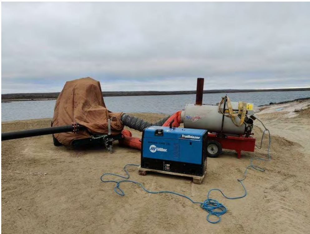
Figure 4-3: Equipment Heater Covering Pump System for Ice Melting
