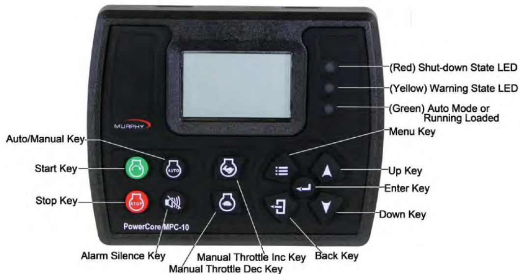
Figure 4-1: Descriptions of Engine Control Keypad
