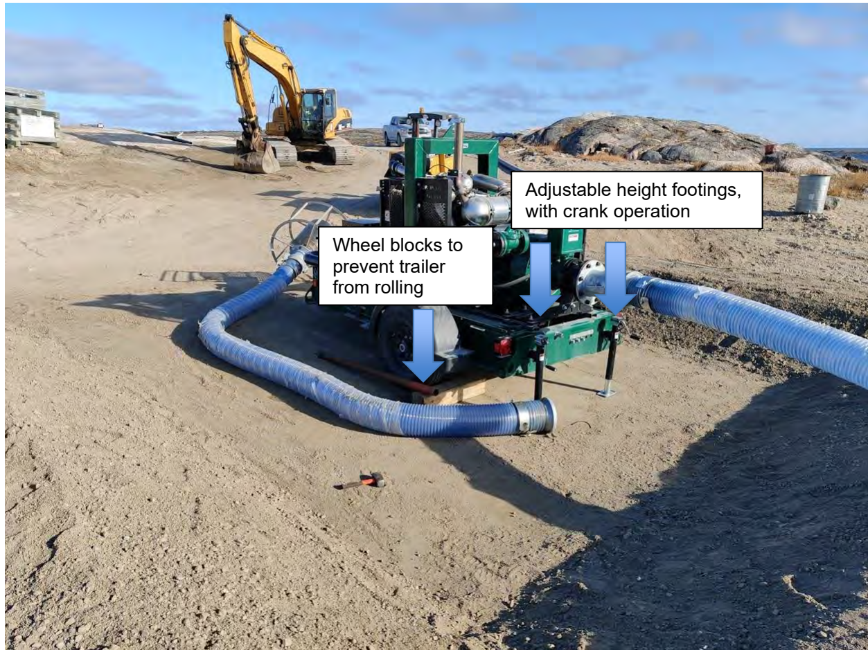
Figure 3.6: Pump Trailers with Footings and Wheel Blocks
