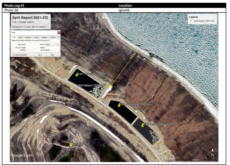
Map of the 3 sewage lagoon cells. Spill Report 2021-372 shows location, and proximity to ocean. A measure of distance from suspected source to ocean measured at 405.41 metres.
