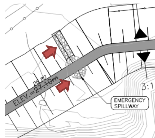
Riprap Upstream Slope - Details
