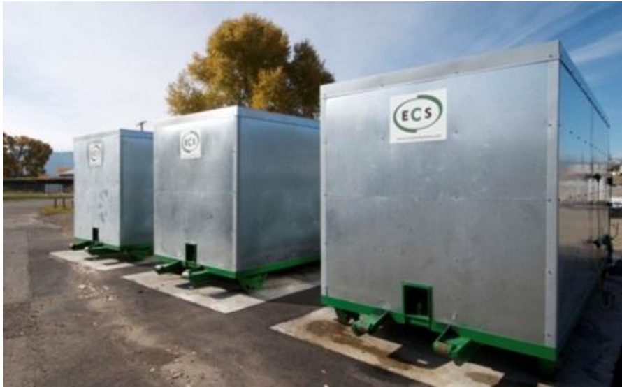
Figure 5: Example of In Vessel System (CV Composter, Engineered Compost Systems, Seattle, WA)
