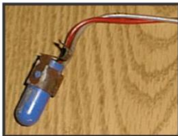
Figure 19: Washing Machine Mercury Switch
