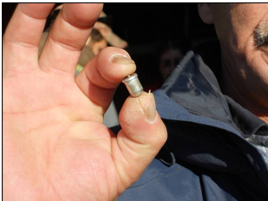
Figure 16: Mercury Pellet removed from Vehicle Convenience Light
