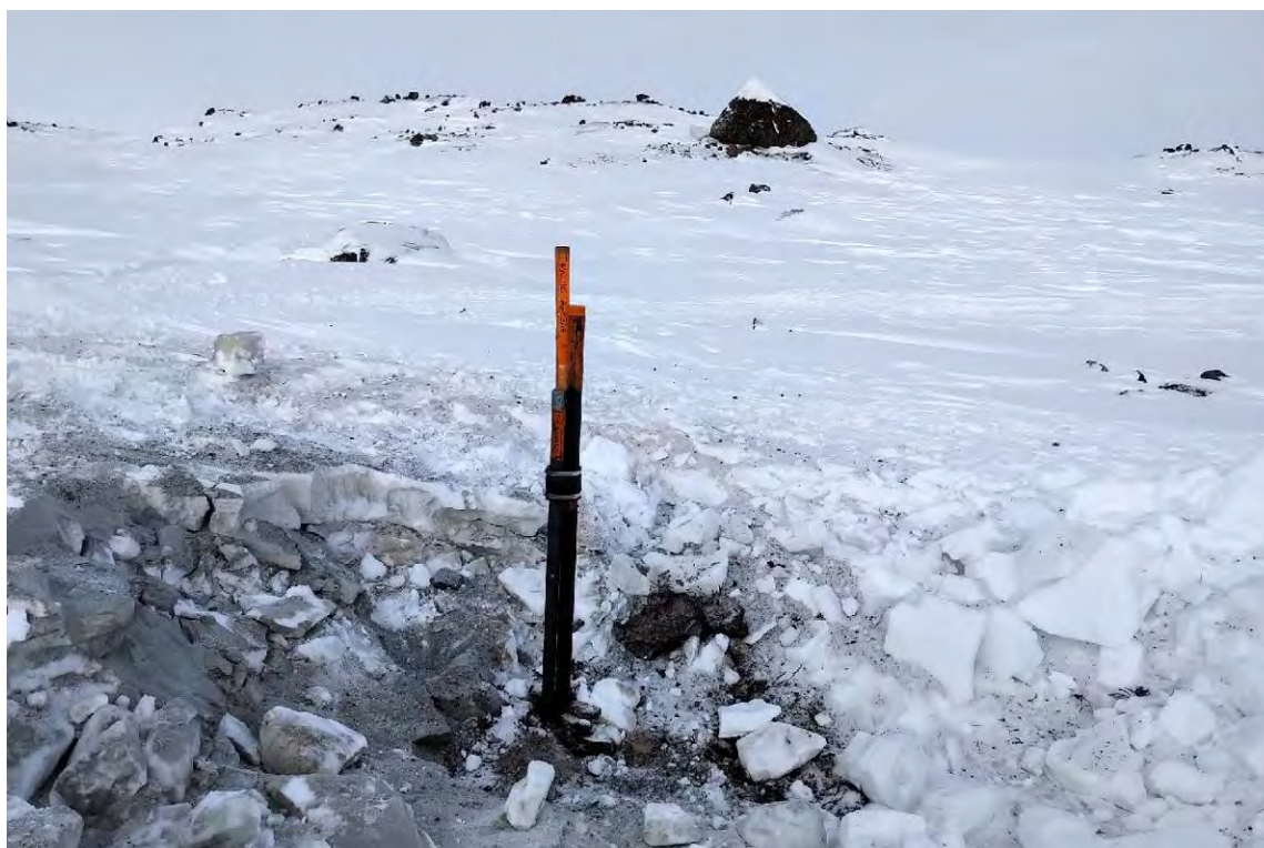
Photo 4 – Temperature and Groundwater Monitoring Installation in TH110/W-110 (Typical)
