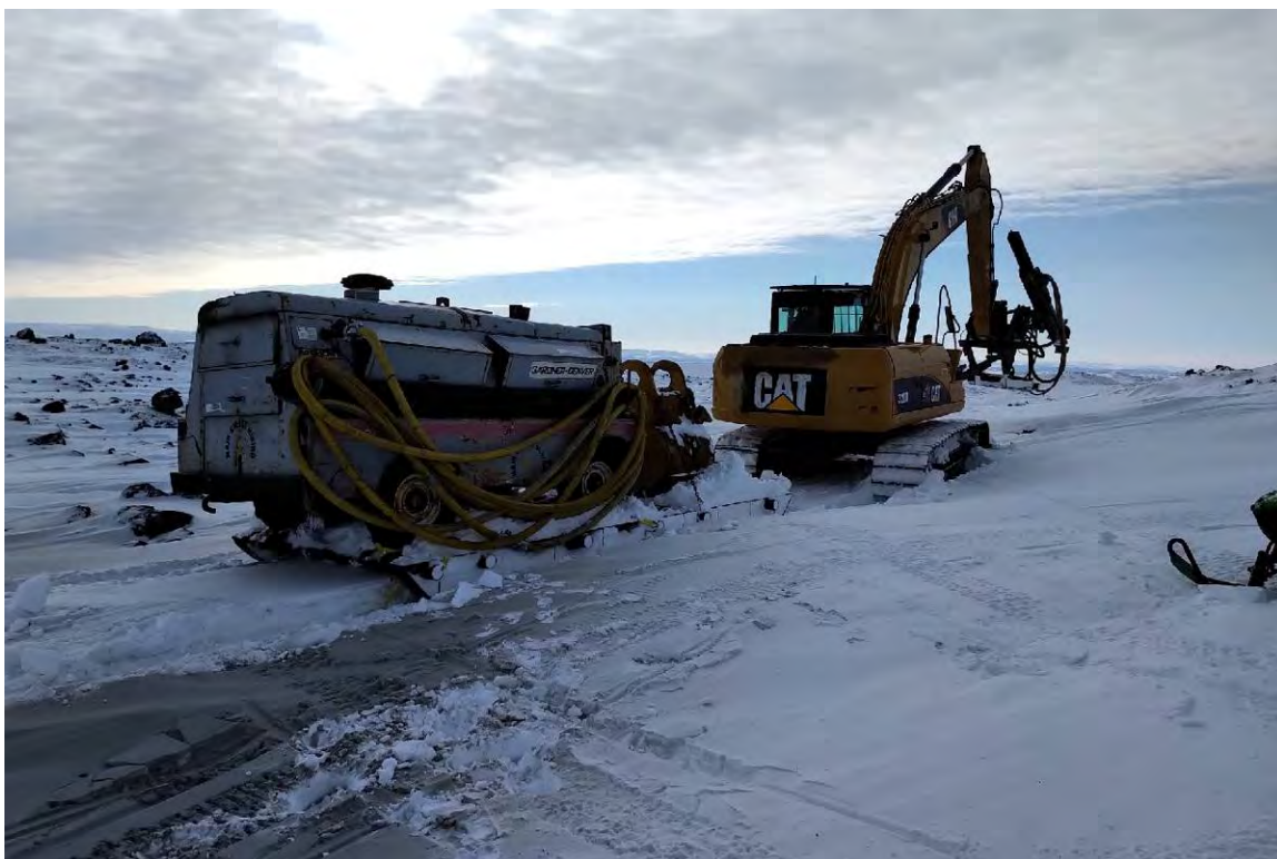
Photo 1 – Typical Air Track Mounted on a Mechanical Shovel and Compressor
