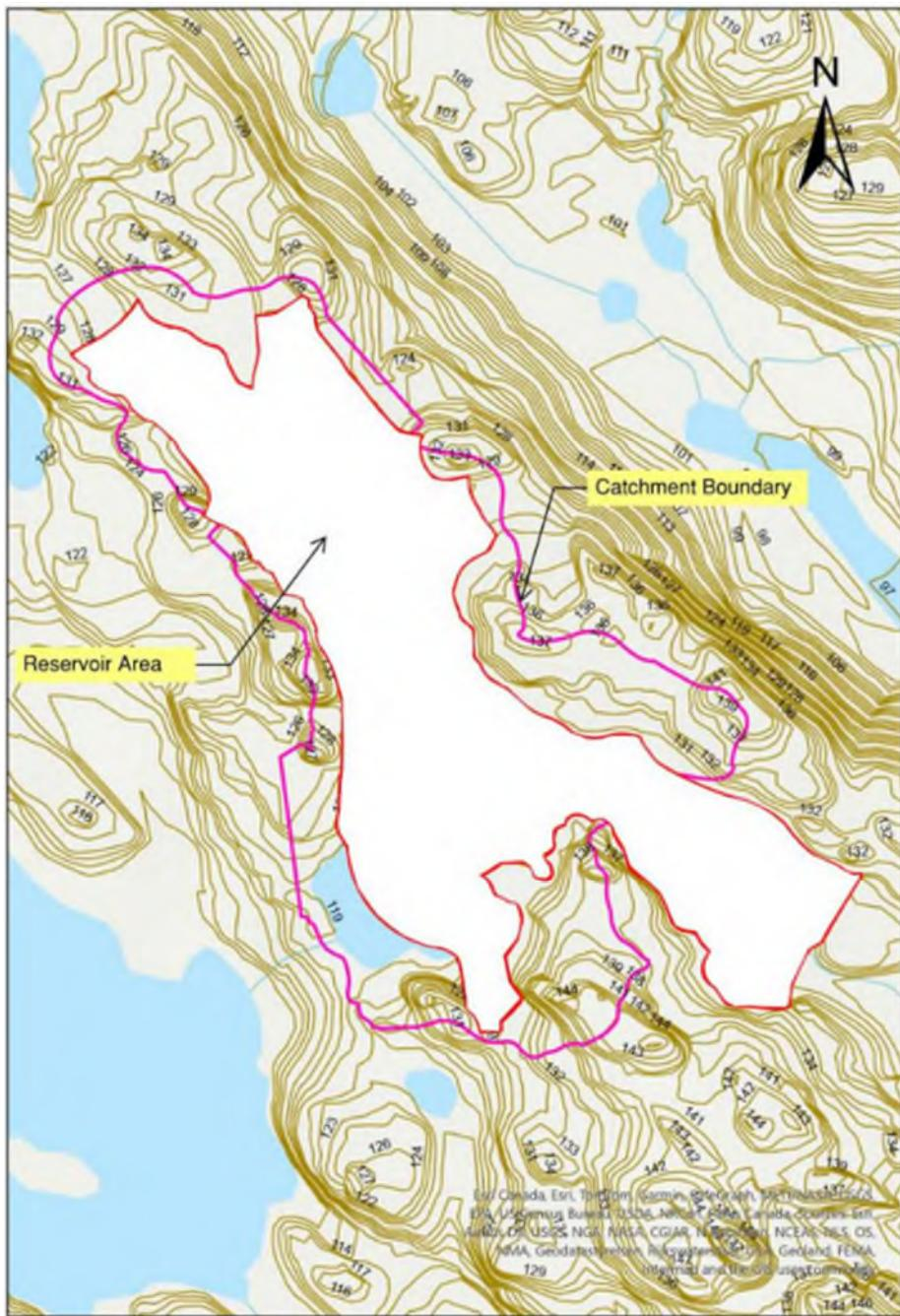
Delineation of the watershed of the Lake Qikiqtaлиk was undertaken by Golder (2021). The total catchment area of Lake Qikiqtaлиk was determined to be 748 ha (7.48 km<sup>2</sup>) with five sub-catchments identified. These are delineated in Figure 2-4.
