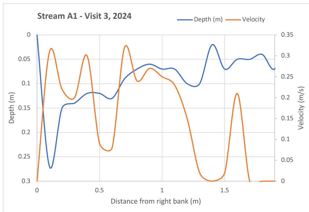
Figure 4. Swoffer flow metering and water depth at site SA1, October 2, 2024.
