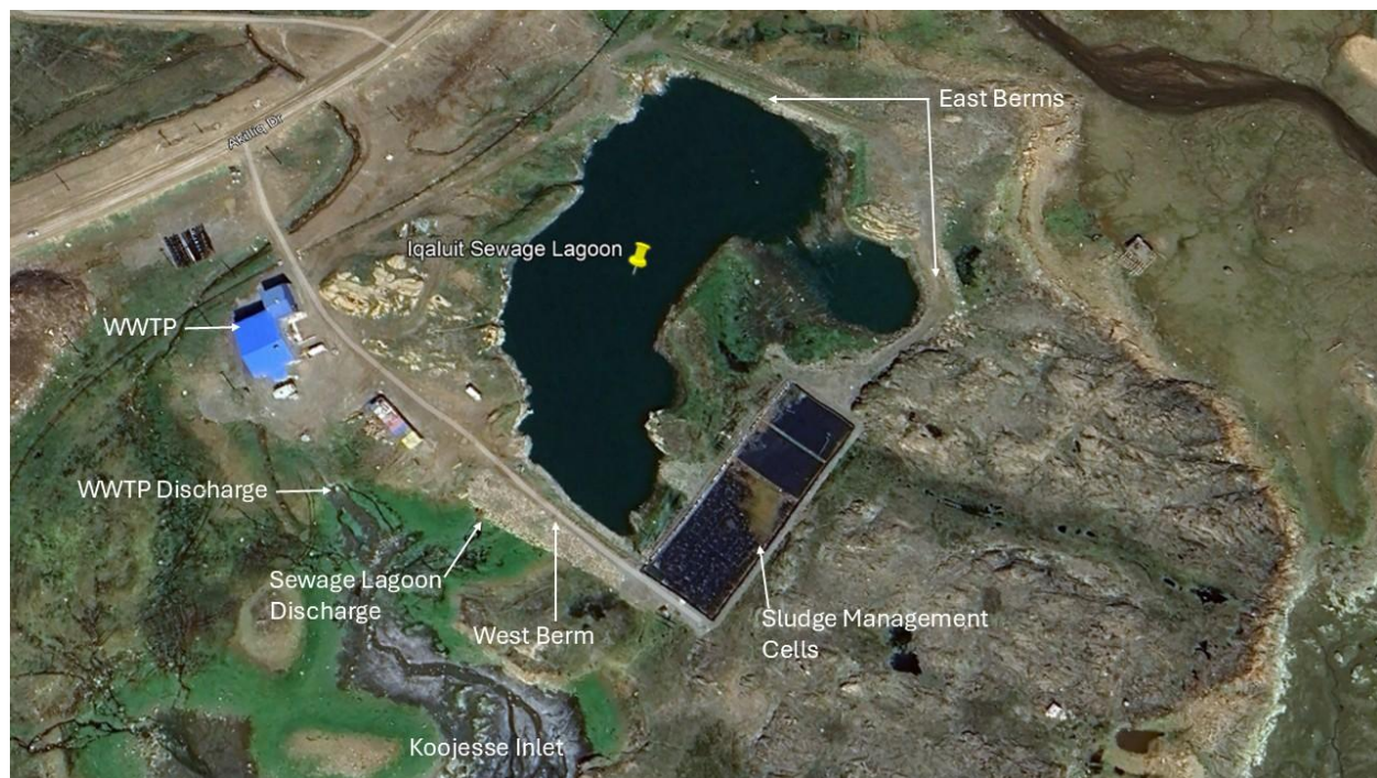
Figure 4.1 Sewage Lagoon Layout
