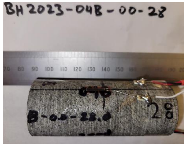
Figure 2: Sample ready for Testing. The rock core sample is prepared with strain gauges and wires, with a ruler for scale showing the length is approximately 85 mm.
