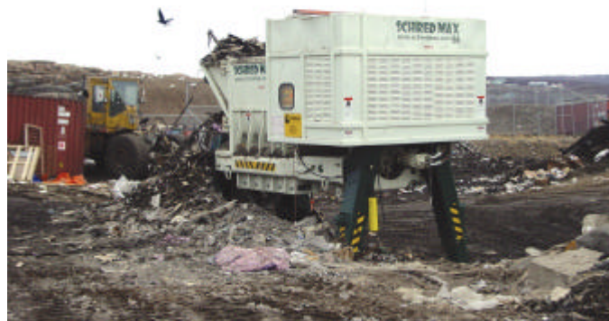
A shredder, used to minimize the volume of waste, in operation at the City’s landfill. Photo credit - Scott Stewart, INAC
