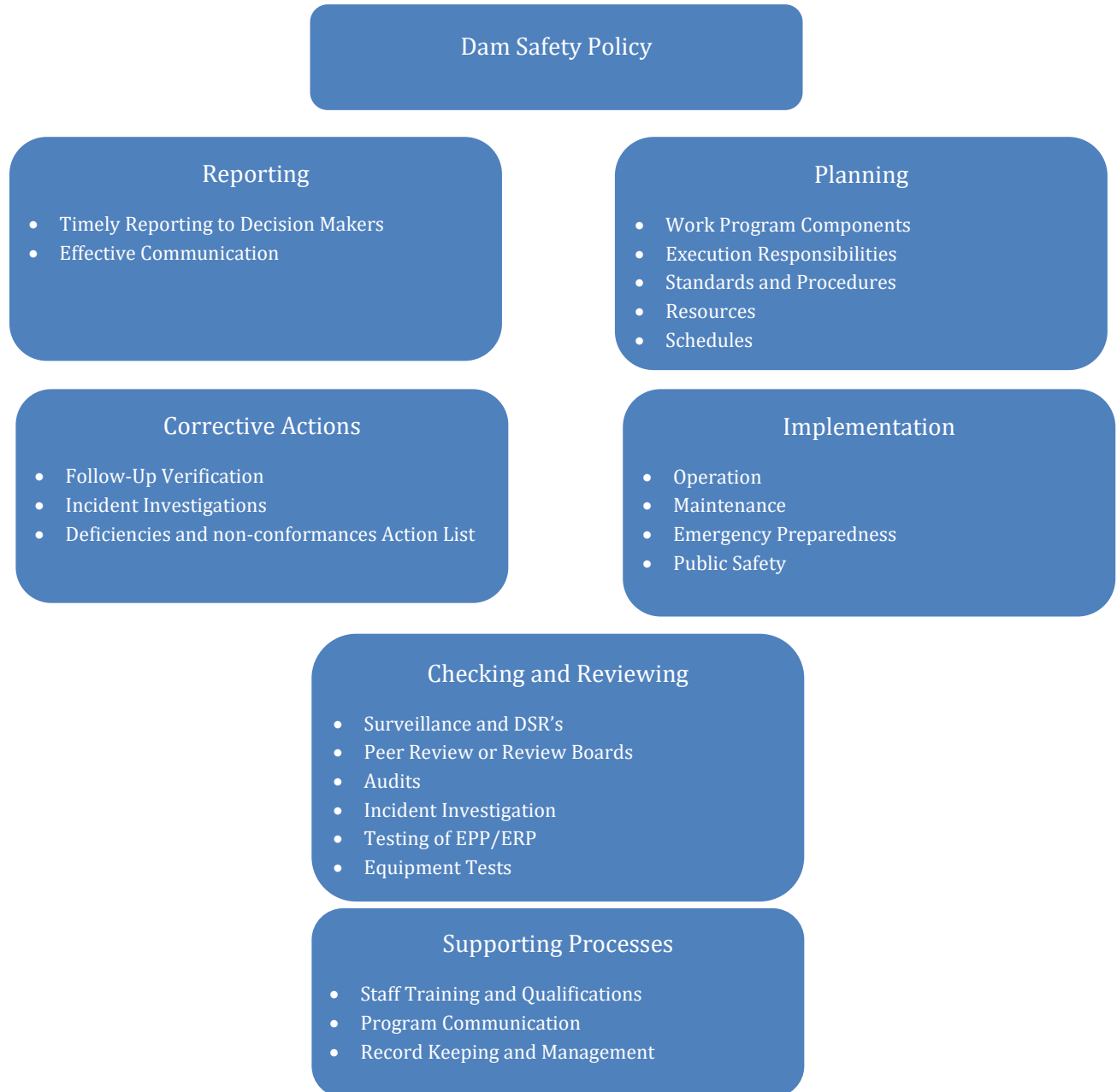
Figure 4.1 Dam Safety Management System (CDA Guidelines, 2013)
