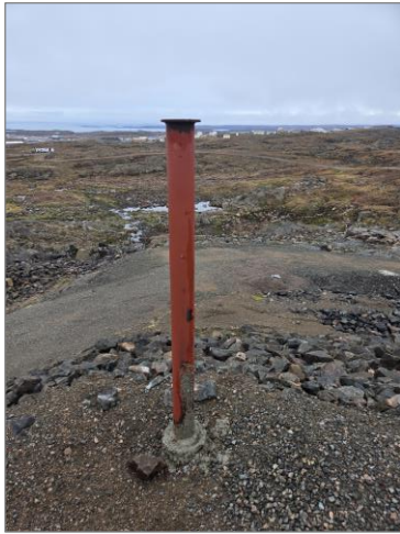
Figure 22 BH107 with Piezometer
