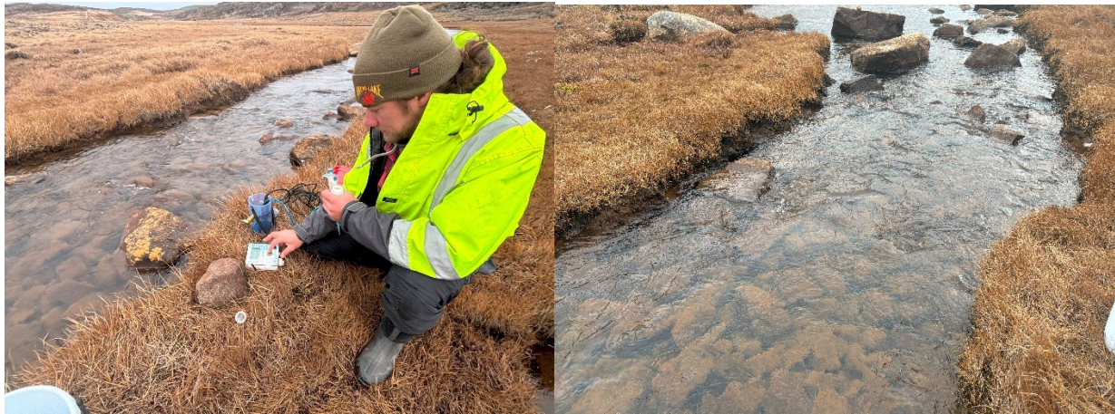
Figure 18. Site Overwinter LL2. (Left) AAE Tech employee using the QiQuac to take flow measurement; (Right) Looking downstream just past where the measurement was taken.
