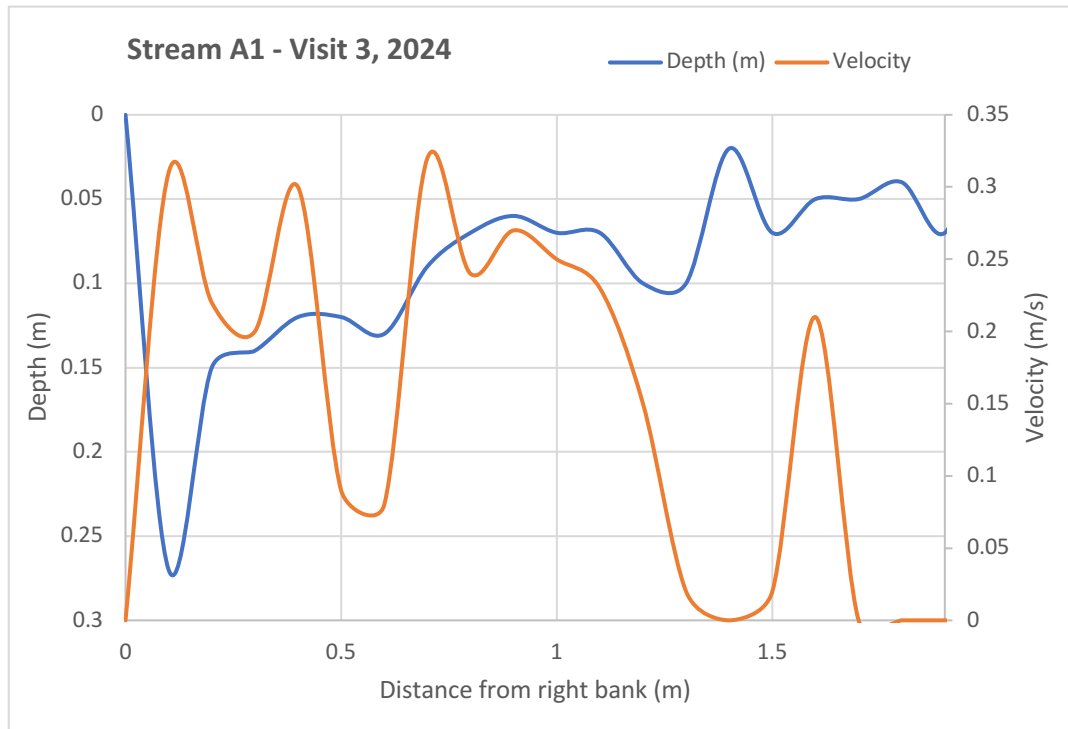
Figure 4. Swoffer flow metering and water depth at site SA1, October 2, 2024.
