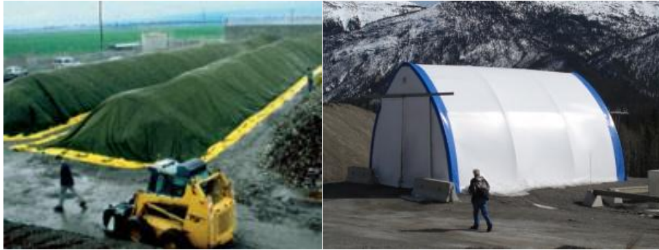
Figure 7: Covered Windrow (left); tension fabric structure (right).
