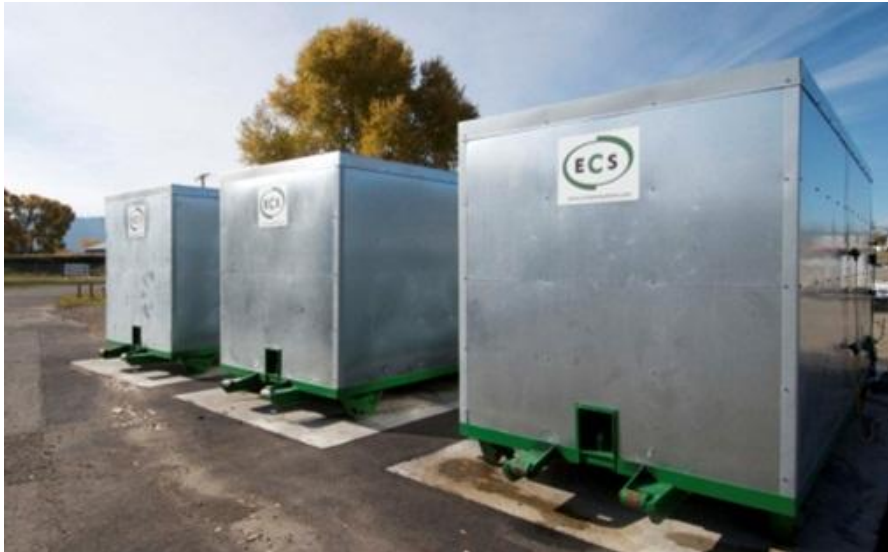
Figure 5: Example of In Vessel System (CV Composter, Engineered Compost Systems, Seattle, WA)
