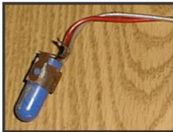
Figure 19: Washing Machine Mercury Switch
