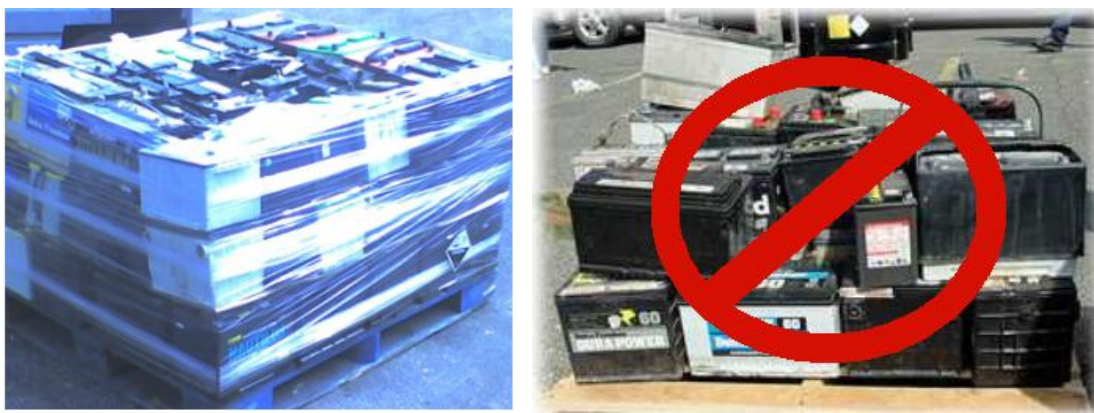
Figure 2 – The Proper and Improper Storage of Lead-Acid Batteries Source: Transport Canada
