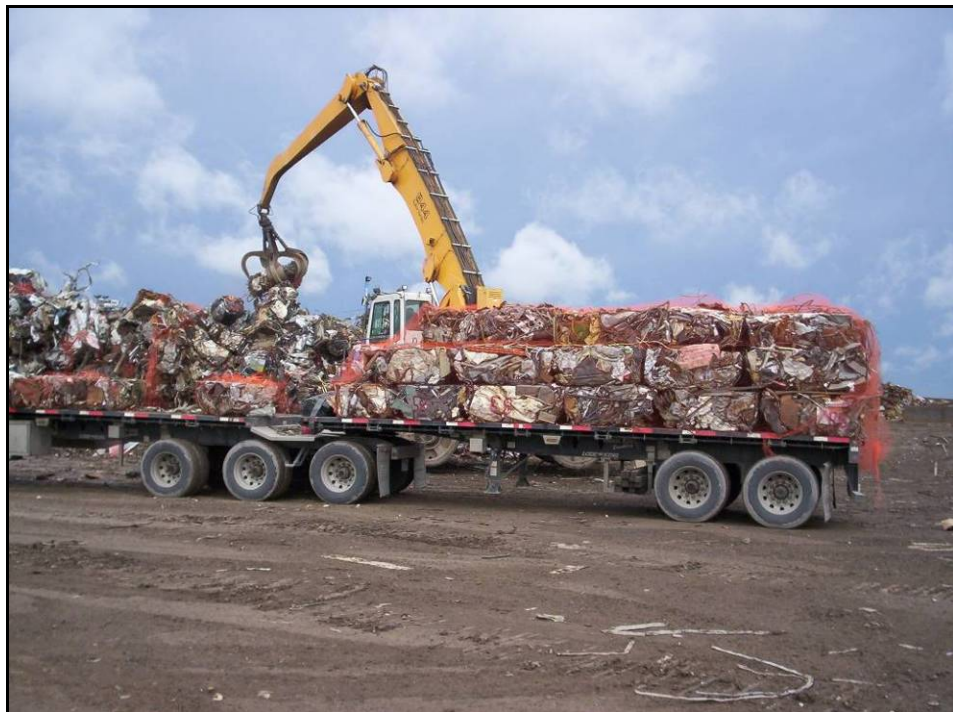
Figure 6: Example of "Logged" Metal
