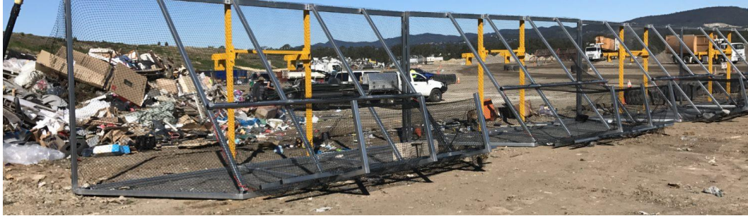
Litter screen positioned down wind of tipping face, near the tipping face. As wind direction changes screens portable require re-positioning. Photograph courtesy of Contained Waste Solutions
