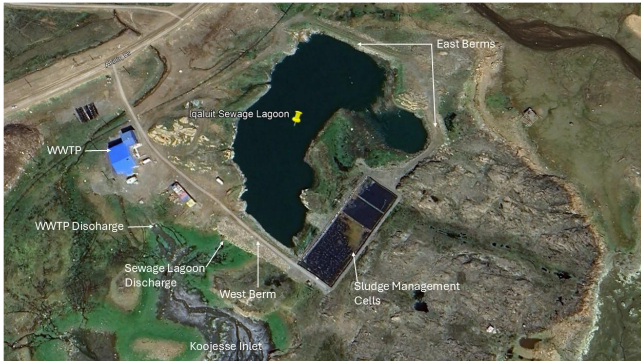
Figure 2 Layout of Sewage Lagoon and WWTP
