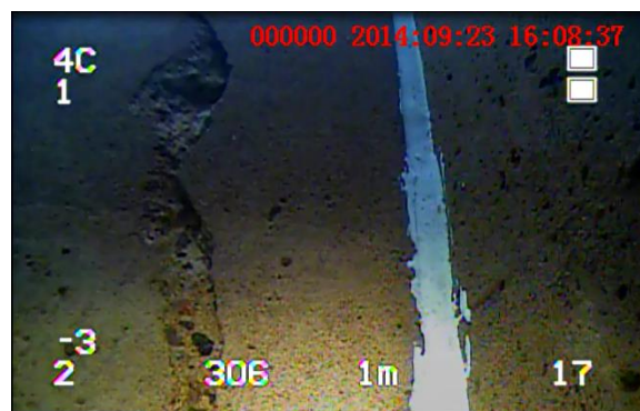
Figure 3-7: Spalling a metre or so below spillway crest to left of J1.
