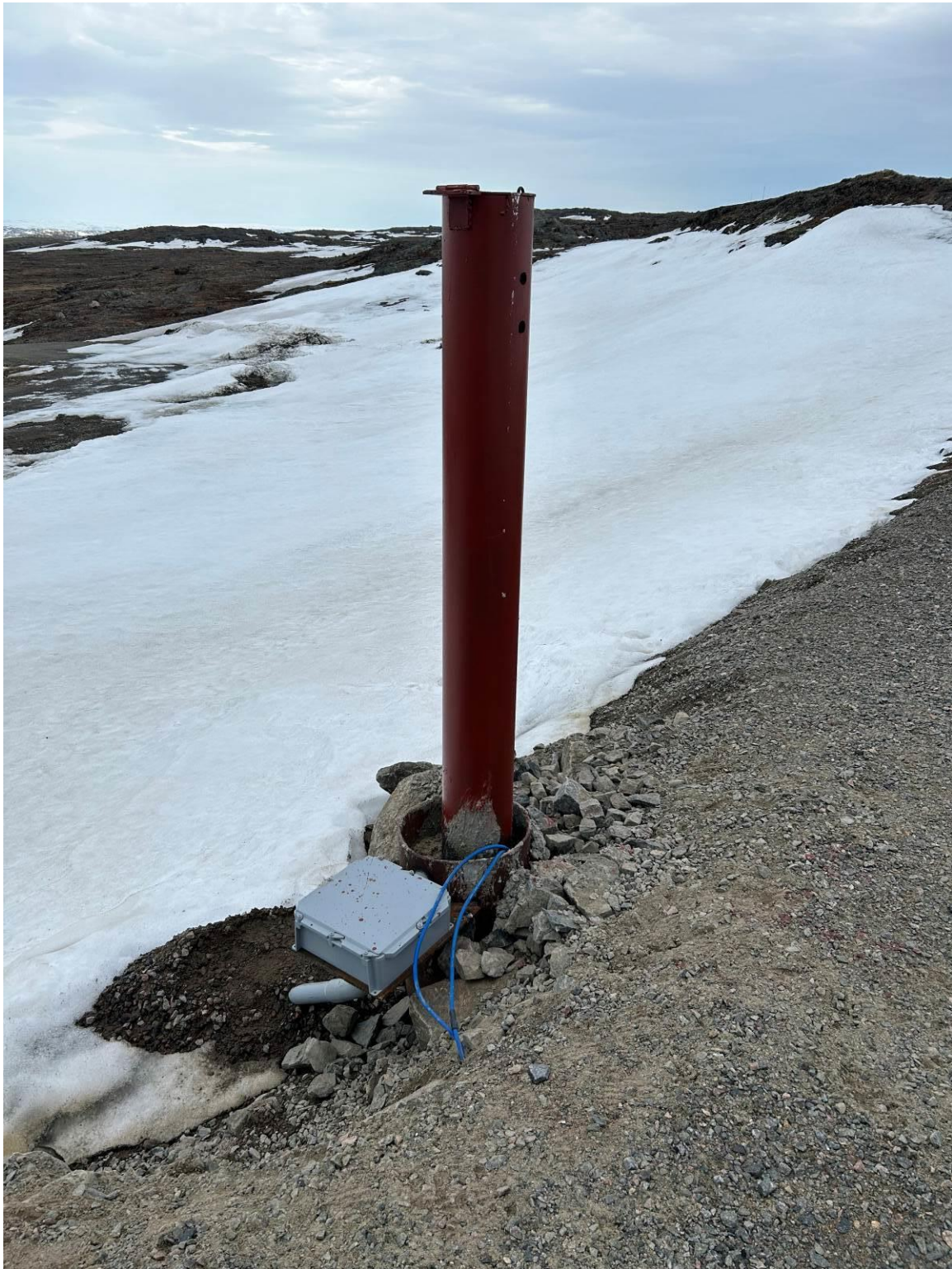
Photograph 10 – Typical temperature data logger installation.
